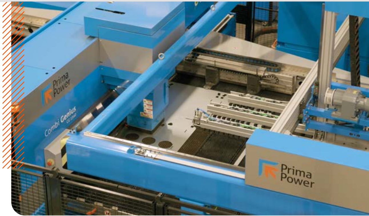
The Combi Genius CG 1540 combines punching and laser cutting.
