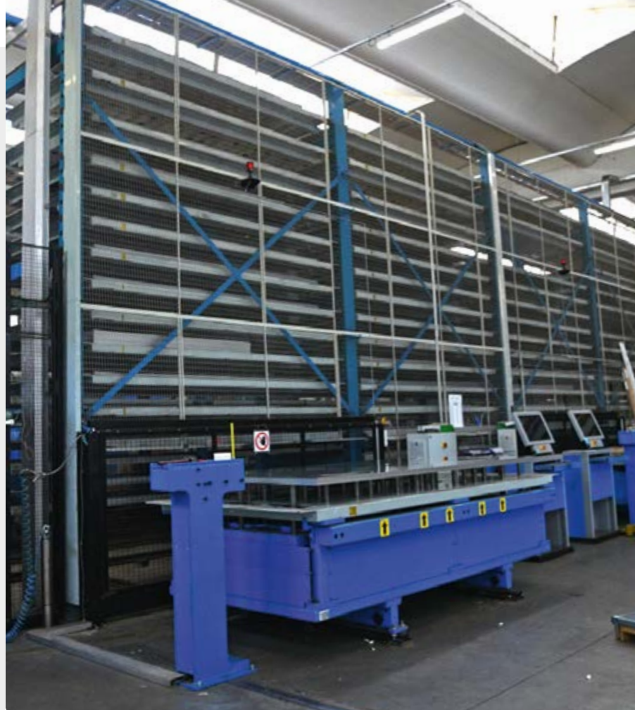
Rizzato's automatic storage system has been updated and extended twice in 20 years and is currently connected to five Prima Power cutting machines.
