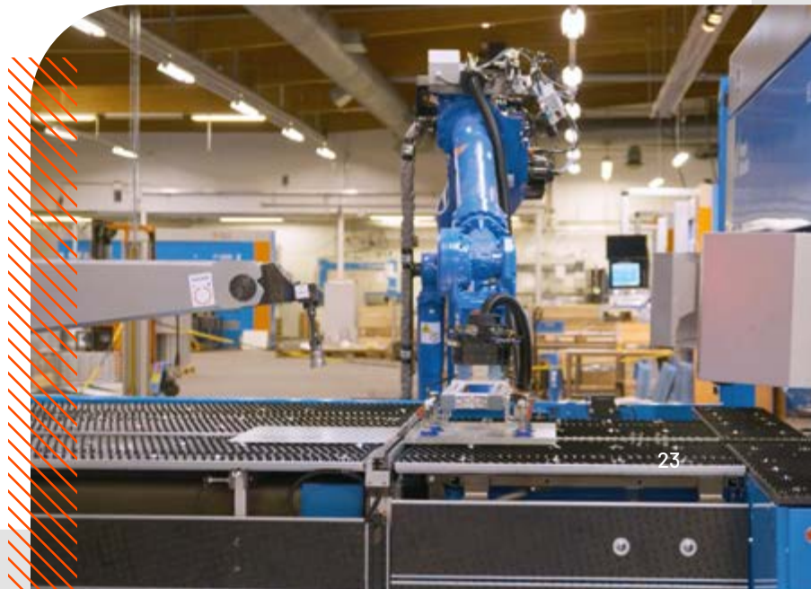
The panel bender installed at Stremet is equipped with a robot to handle loading and unloading.
