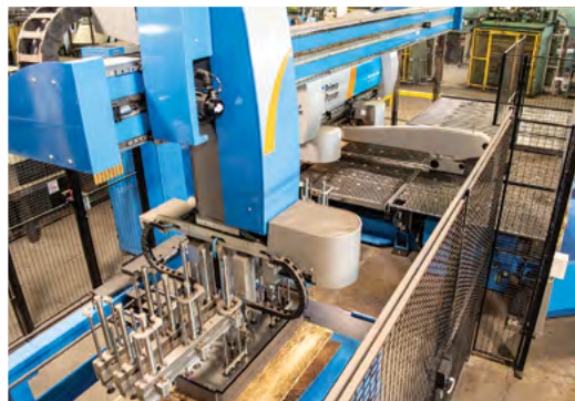
The bending operation is fully automated, from the loading of flat punched parts to unloading of the finished product.
