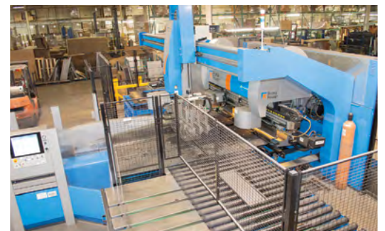
The EBe servo-electric panel bender is a bending solution that is designed specifically for each fabricator's production requirements to achieve maximum productivity, quality, and repeatability.
