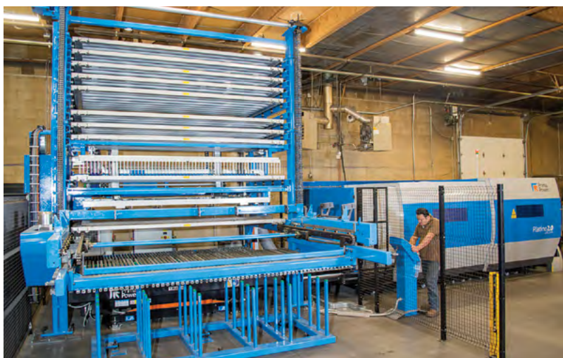
Precision Laser Processing utilized its existing Prima Power 10-shelf TowerServer automated work handling system for the 4 kW Platino Fiber (above) and purchased a new 10-shelf tower for the 6 kW model (left).
