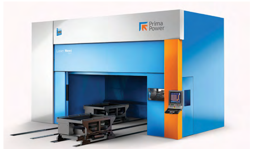
Movable table configuration with manual or automatic movement, both in X or Y direction.
