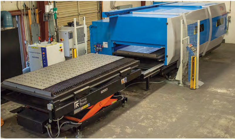
The Prima Power Platino Fiber has doubled the cut production in making parts at Metal Werks while increasing the company's quality.
