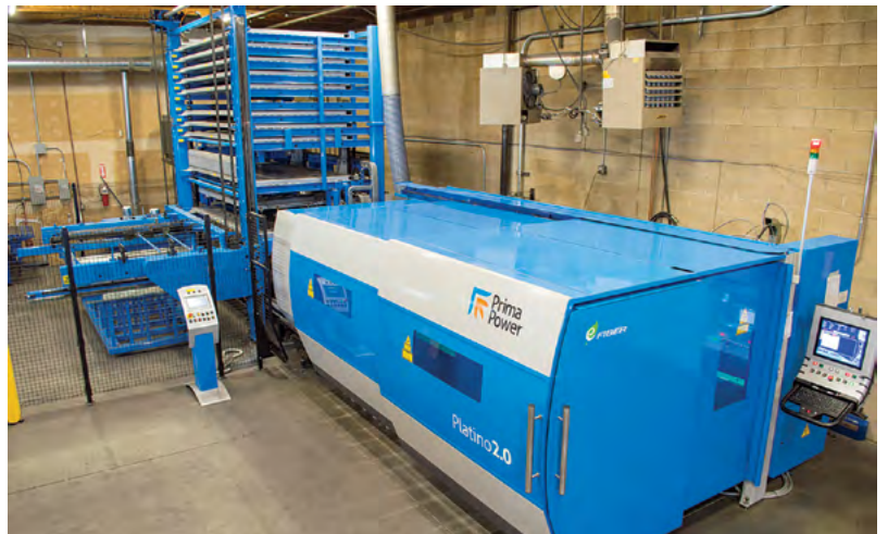
Precision Laser Processing utilized its existing Prima Power 10-shelf TowerServer automated work handling system for the 4 kW Platino Fiber (above) and purchased a new 10-shelf tower for the 6 kW model (left).
