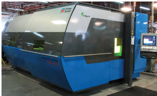
The Prima Power Sincrono Fiber laser features 6g acceleration for processing thin sheets.
