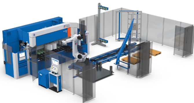
Fast Bend panel bender with 7-axis robot
