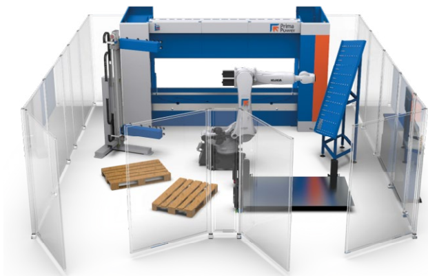
eP press brake with 6-axis robot
