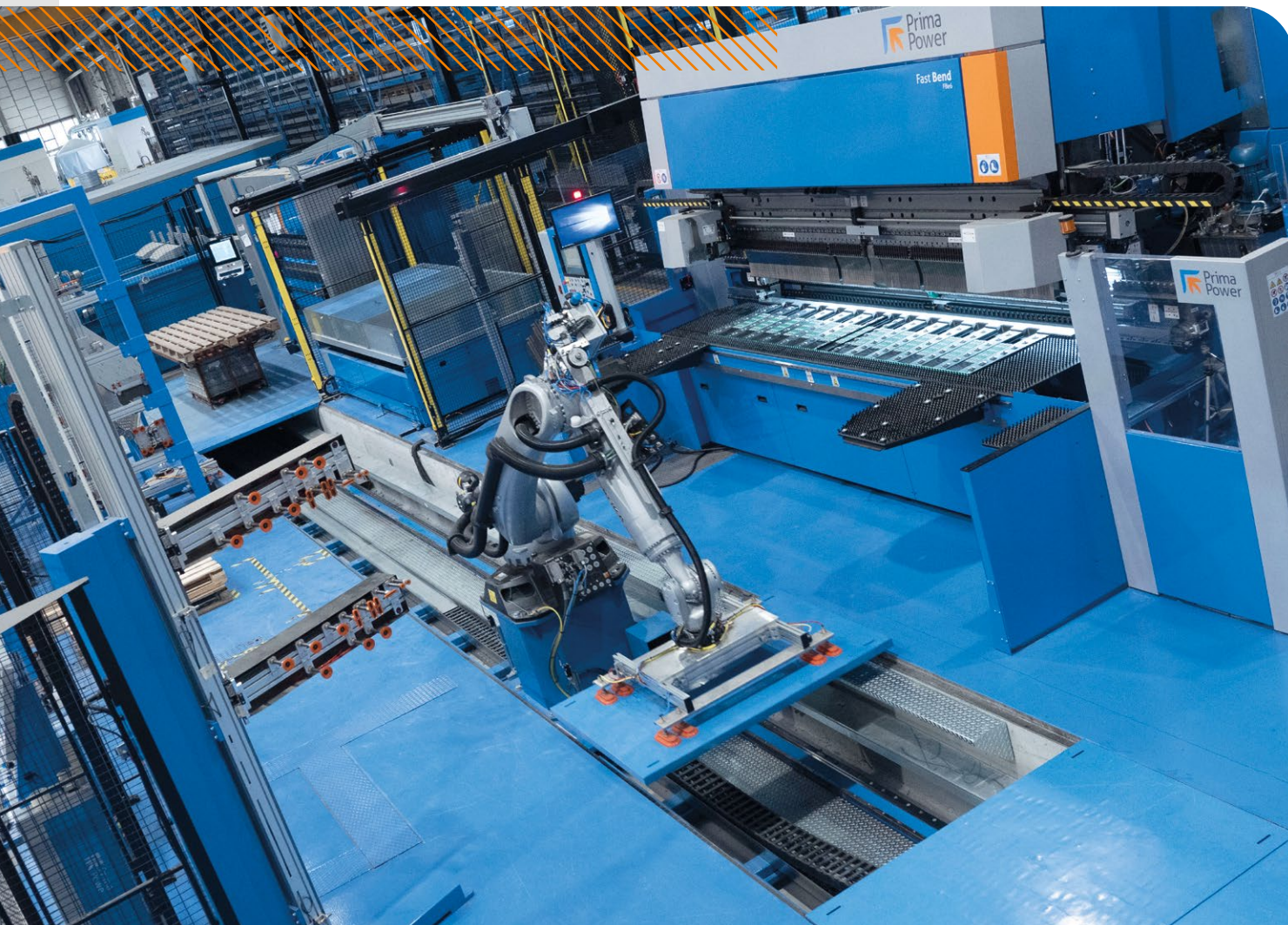
The robot moves on the front of the machines along its 19 m track, which allows it to cover both the bending machine and the panel bender as well as the three unloading bays.
