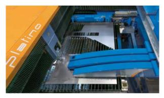
Platino equipped with LST for part sorting and stacking.
