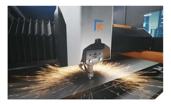
Best-in-class dynamics to grant low cycle times with excellent cutting quality. Laser Genius<sup>+</sup> can process with high quality levels a wide range of materials up to 30mm and can be equipped with laser generator with powers ranging from 2 to 15 kW.
