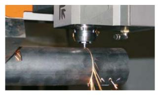
Platino easily switches to tube cutting.
