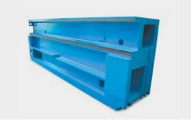
Synthetic granite frame provides top mechanical rigidity and stability.
