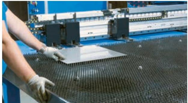
Smaller sheets are positioned against the third and fourth loading pin.
