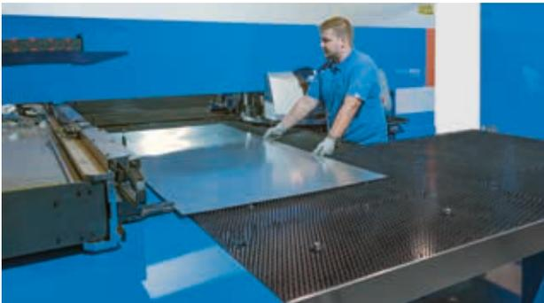
Larger sheets are positioned against the first and second loading pin.
