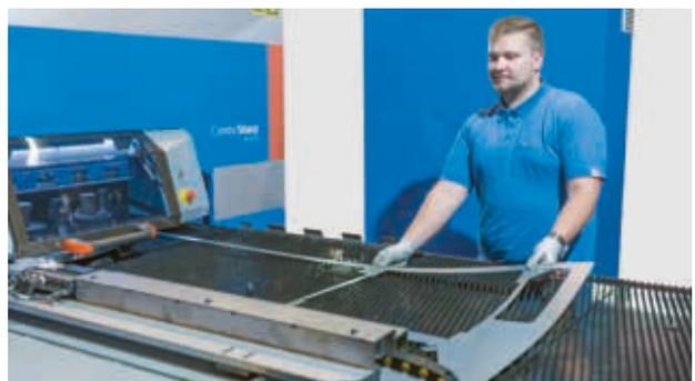
Skeletons can be removed from either side of the machine.
