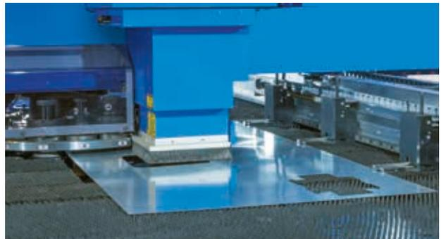
Laser cut parts up to 500 x 500 mm (machine size 1225) or 300 x 400 mm and 800 x 800 mm (machine size 1530) are dropped through the door in the table onto conveyor below.
