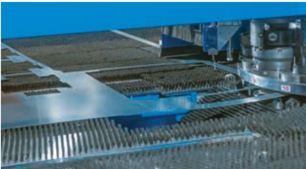
Punched parts up to 500 x 500 mm are dropped through the door in front of the turret for separate sorting.
