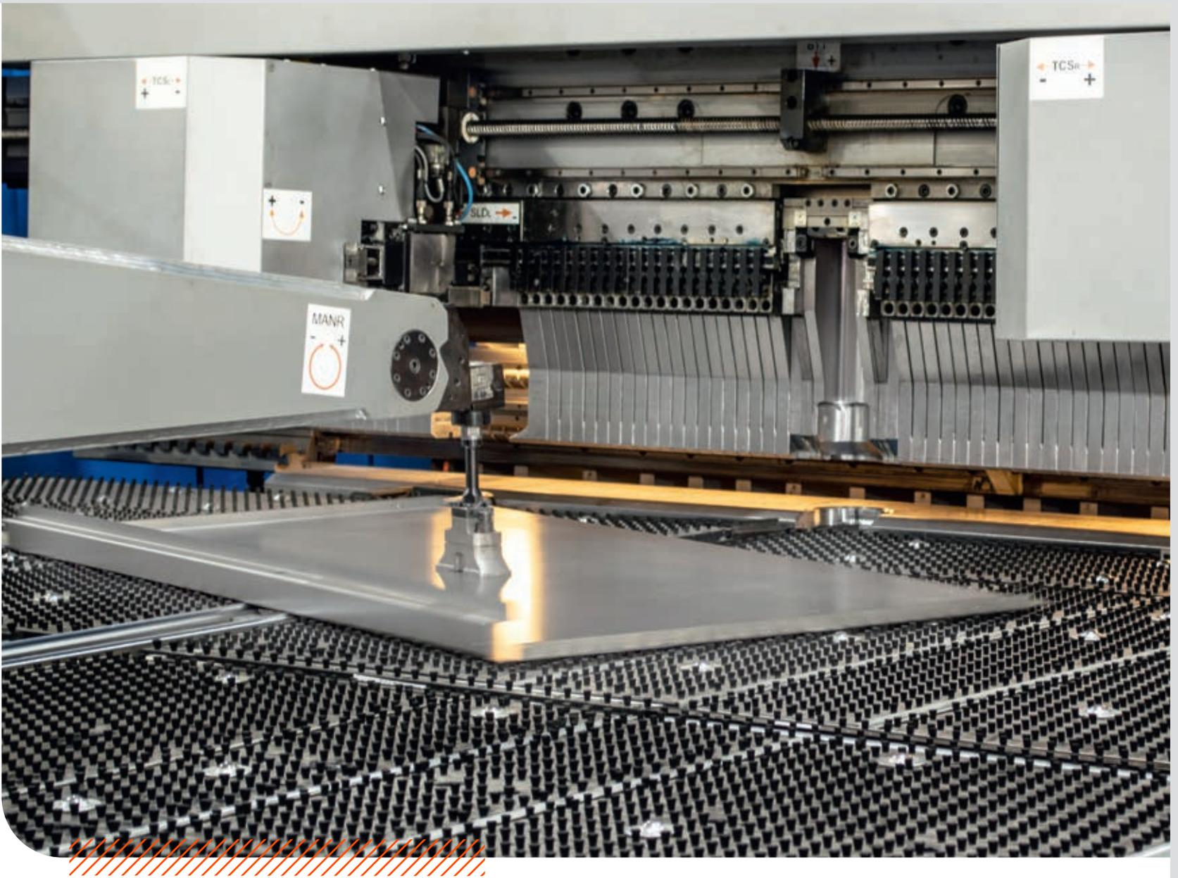
The Prima Power BCe Smart panel-bending machine is integral to FlexMet's efforts in launching its own product lines.
