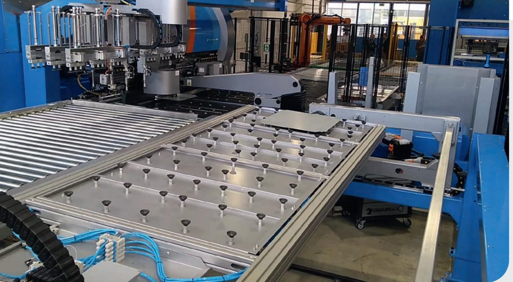
The automatic bending system installed at Schulthess consists of a servo-electric EBe4FM panel bender, an eP0520 press brake, a 7-axis industrial robot sliding on rails, and one palletized conveyor area with automatic pallet feed. Here, a part is being overturned by the EBe's Bending Turning Device for centering on the Picking & Centering Device.
