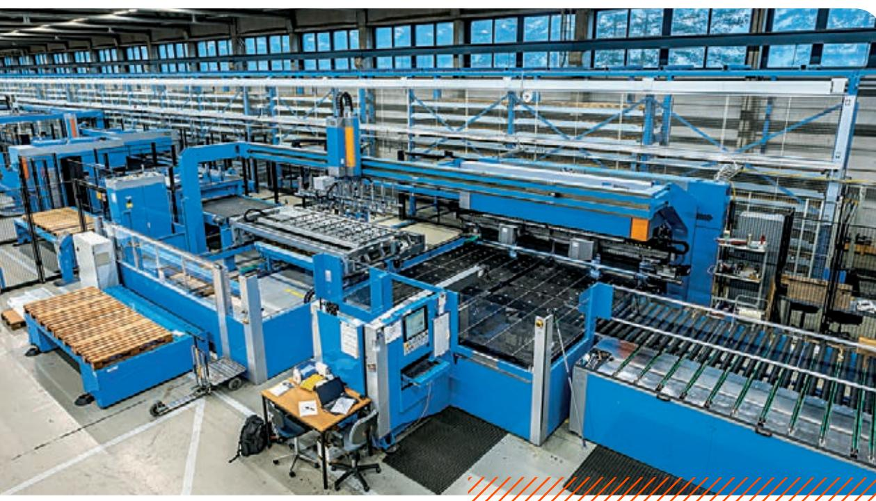
Prima Power manufacturing line connected to the automated storage system Night Train significantly increased Halton's production capacity.
