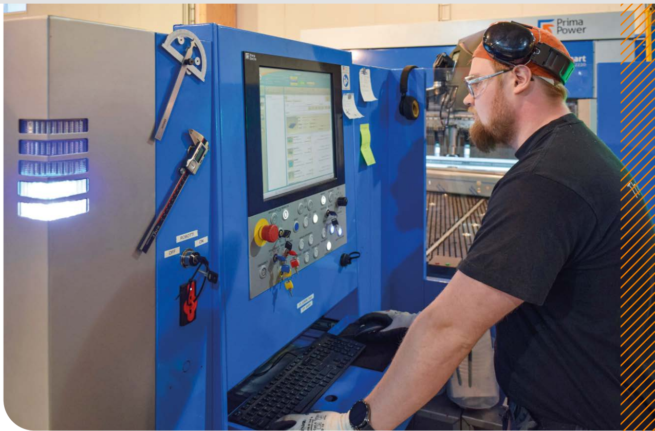
The BCe Smart panel bender offers a bending length of 2250 mm. Toni Pitkänen operating the machine.
