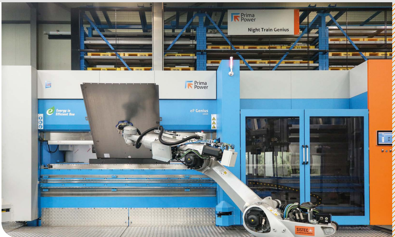
The eP Genius 1030 press brake with automatic tool change storage and 7-axis anthropomorphic robot installed at WOOJIN PLAIMM.
