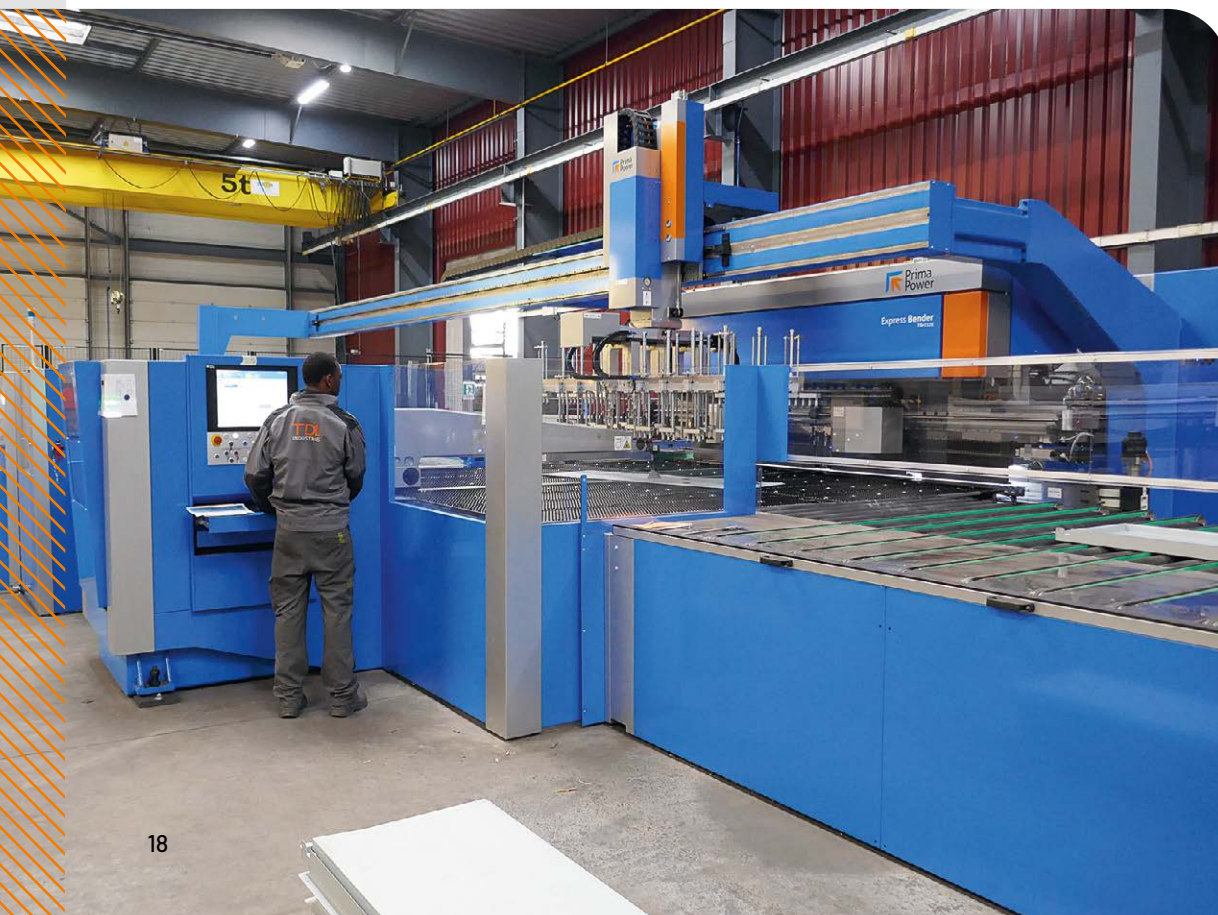
The Express Bender EBe 3320 panel bender installed at TDL Industries is equipped with an automatic loading system. Courtesy of Tôlerie
