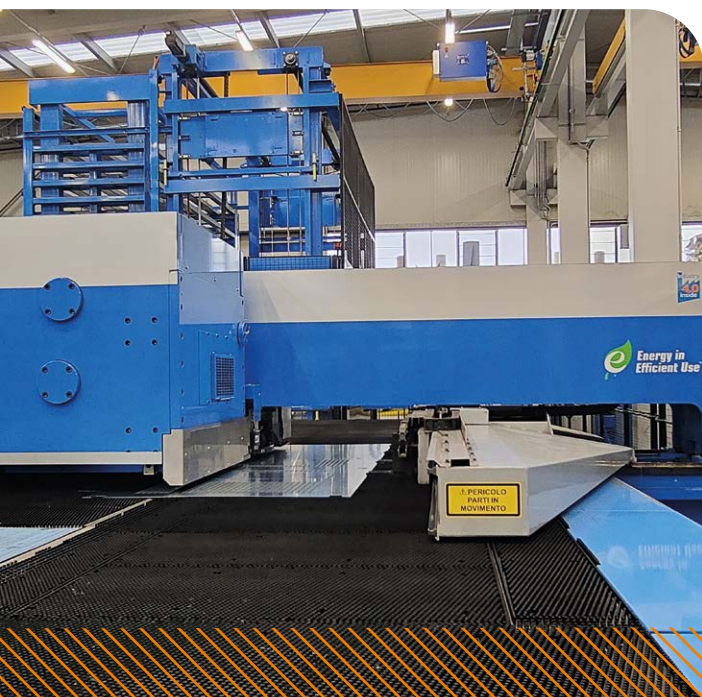
The punching unit on the PSBB line performs multiple processing operations, such as threading or forming, on a single station, thereby enhancing the overall efficiency of the production process
