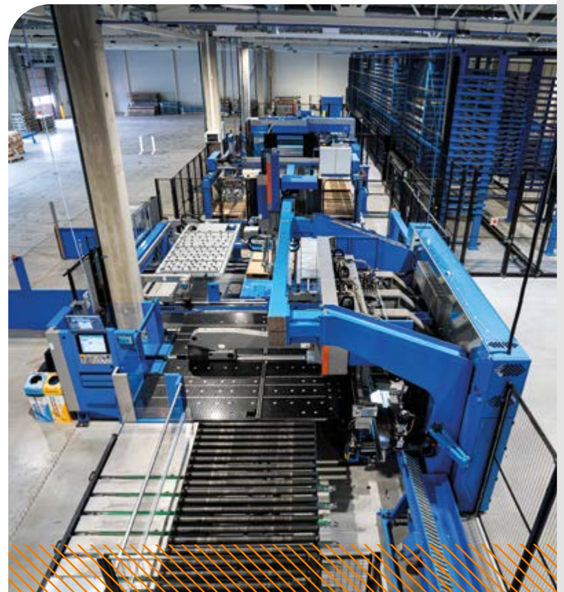
The PSBB (Punching, Shearing, Buffering, and Bending) line runs automatically 24/7, significantly speeding up production processes and increasing output.
