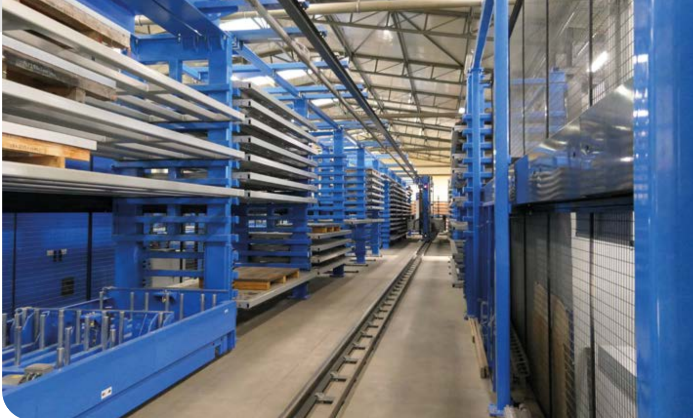
At Alfa 3, the 30-meter Night Train FMS enables complete and flexible automation of the manufacturing process.
