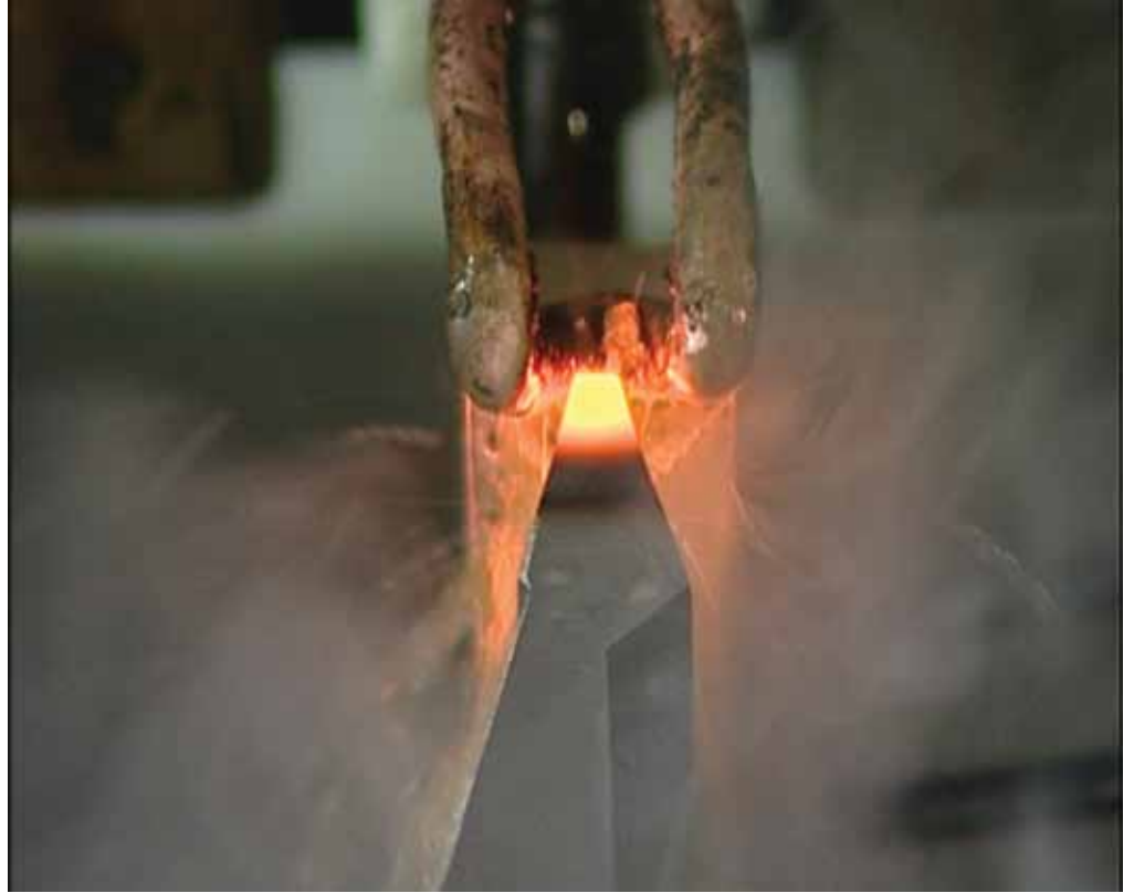
Photograph shows the tip of a Wila Acute-Angle Punch being CNC-DeePhardened.
