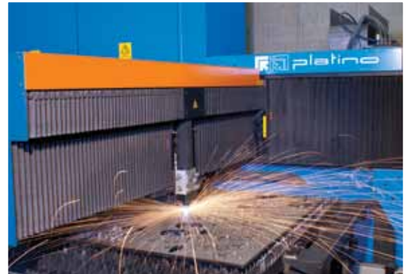
Precision Laser Processing uses the Platino lasers for all material from .001 to 1 inch mild steel plate.
