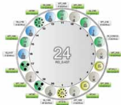
Fig. 3—An electronic tool whiteboard in the machine control alerts the setup operator should the tooling loaded in the turret not match that of the NC program. An easy-to-read screen on the control shows the turret layout along with the tools being used for the current program (in green).
