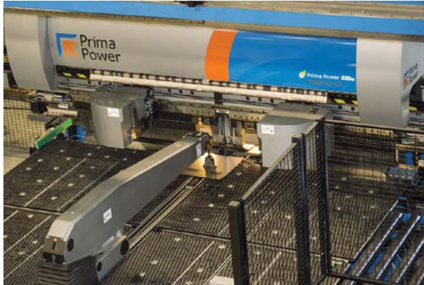
BMP procured the Prima Power EBe panel bender in 2015. The EBe servo-electric Express Bender is a bending solution that is designed specifically for each fabricator's production requirements to achieve maximum productivity, quality, and repeatability.
