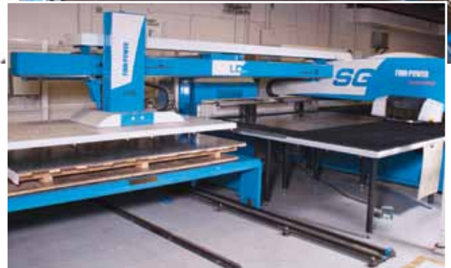
To increase its flexibility and decrease its material handling, Artopex purchased a Prima Power punch/shear/bend cell in 2009. With the Shear Genius integrated punch/right angle shear combination concept, the objective is to provide one machine capable of transforming a full-sized sheet into punched parts.
