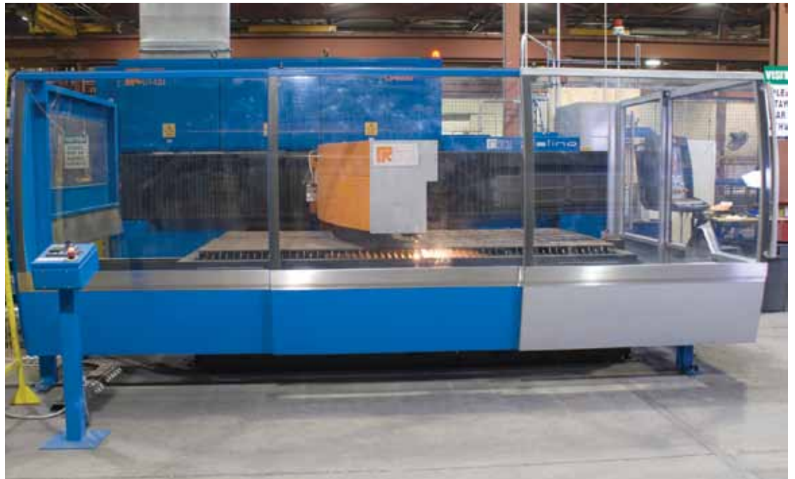
The Platino is equipped with lasers developed and produced at Prima Industrie in laser powers ranging from 3000 to 5000W. The laser cuts a broad range of materials and thicknesses with speed and precision without the need for manual adjustments.
