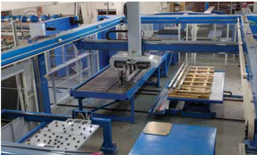
The Prima Power flexible manufacturing system includes the Express Bender (EBe5) automated bender, seen in top image, and the Shear Genius (SG) punch/shear combination machine, seen below in the background, with transfer table in forefront.
