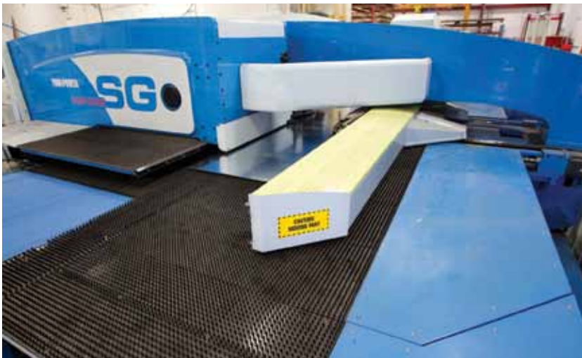
The Shear Genius (SG) integrated punch shear combination transforms a full-sized sheet into punched parts.
