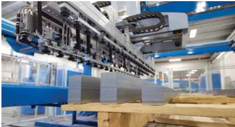
The Sorting and Stacking Robot, seen here, automatically unloads parts from the Shear Genius (SG) and loads them to the Express Bender (model EBe5) automated bender.
