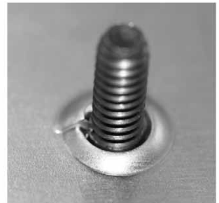
Photo shows the completed form, with a 10-24 machine screw.
