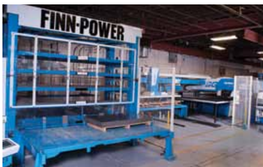
To increase its flexibility and decrease its material handling, Artopex purchased a Prima Power punch/shear/bend cell in 2009. With the Shear Genius integrated punch/right angle shear combination concept, the objective is to provide one machine capable of transforming a full-sized sheet into punched parts.
