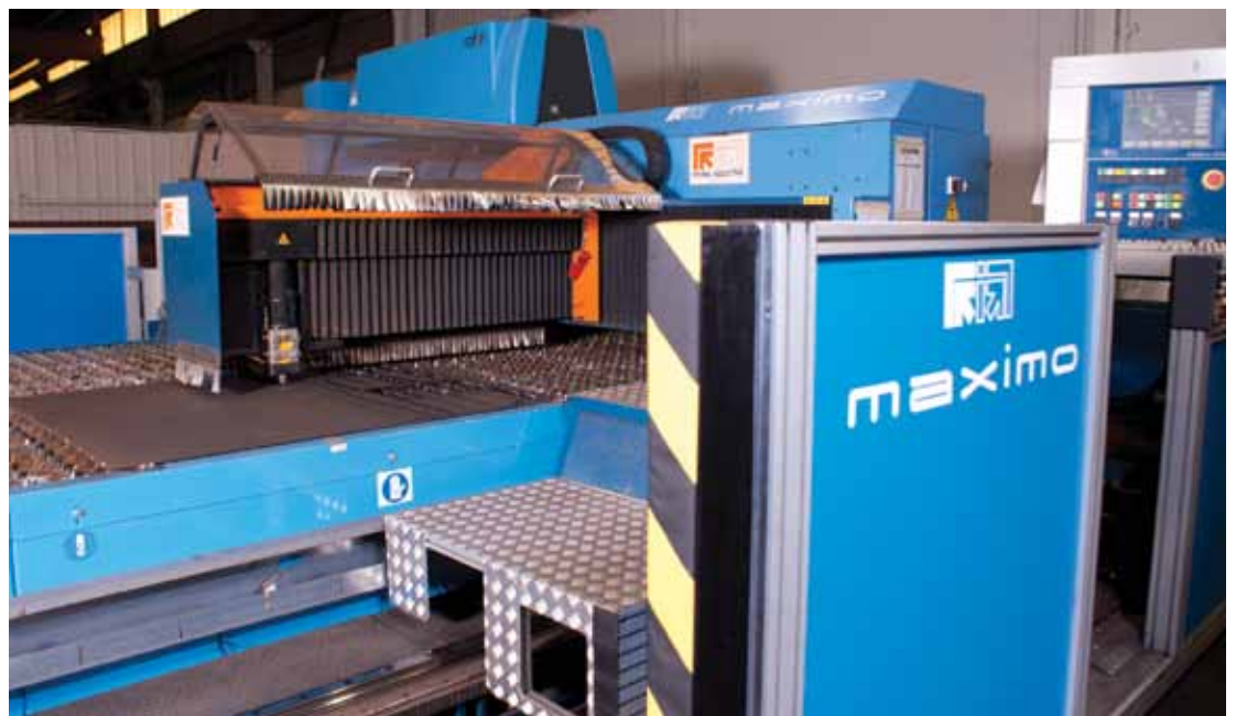
The system is equipped with a platform for the operator, which moves together with the machine. From this position, the operator can have full control of the cutting process, both watching the work area and checking all work parameters on the CNC screen.
