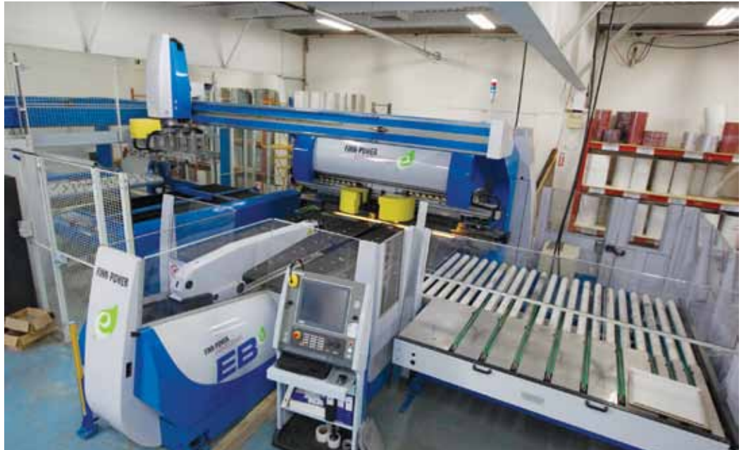
Prima Power's flexible manufacturing system (FMS) has given Lenmak a strong competitive edge. The system includes an automated bender (Express Bender EBe5), seen here.
