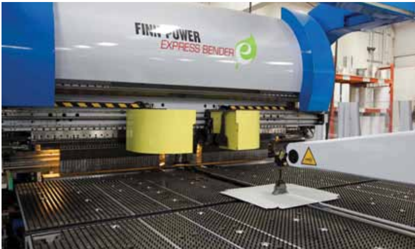
The Prima Power flexible manufacturing system includes the Express Bender (EBe5) automated bender, seen in top image, and the Shear Genius (SG) punch/shear combination machine, seen below in the background, with transfer table in forefront.
