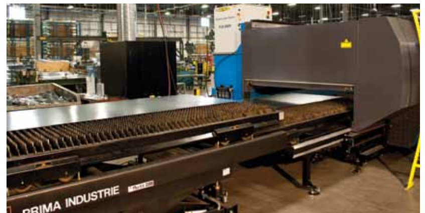
The unique architecture of PLATINO fiber allows full accessibility to the working area from three sides. PLATINO Fiber is available for sheet size up to 1,500 x 3,000 mm and with laser power ranging from 2,000 W up to 3,000 W, and is suitable for a wide range of applications.
