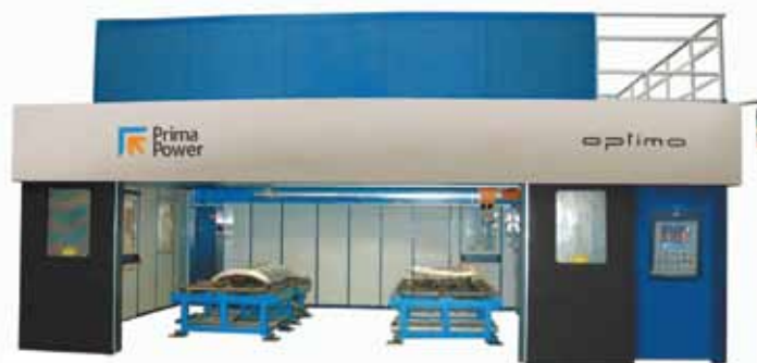
Optimo, the 3D laser machine by Prima Power used to cut and weld the 2012 Olympic Torch
