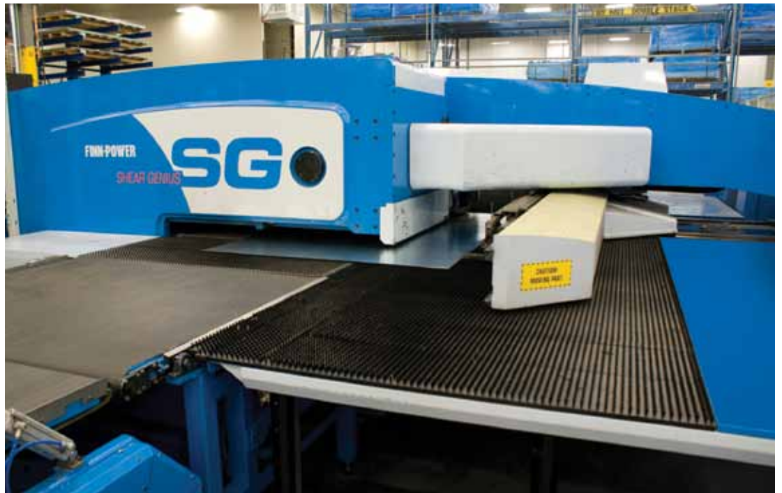
The same clamps that hold the sheet for punching also hold it for shearing. In essence, the Shear Genius allows the automated process to begin with a full-sized sheet of material and end with a punched part.
