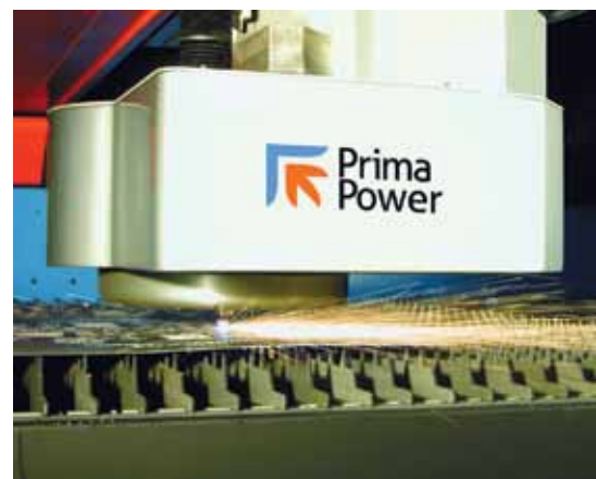
Sincrono, the 2D laser cutting machine by Prima Power used to cut holes on the Torch
