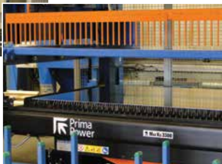
While the parts are being laser cut, the Compact Tower positions the next sheet on the waiting sliding table. Once the first sheet is finished, the tables switch over, minimizing idle time, cutting then resumes and the completed sheet is stored in the tower.
