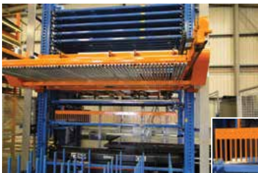
While the parts are being laser cut, the Compact Tower positions the next sheet on the waiting sliding table. Once the first sheet is finished, the tables switch over, minimizing idle time, cutting then resumes and the completed sheet is stored in the tower.
