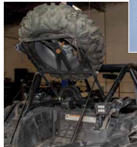
Prior to opening his job shop, Larry Rosevear honed his sheet metal fabrication skills by building dune buggies. Today, Laser Innovations services a wide variety of industries, however, he still makes some dune buggy parts such as this spare tire hydraulic auto-assist power mount.
