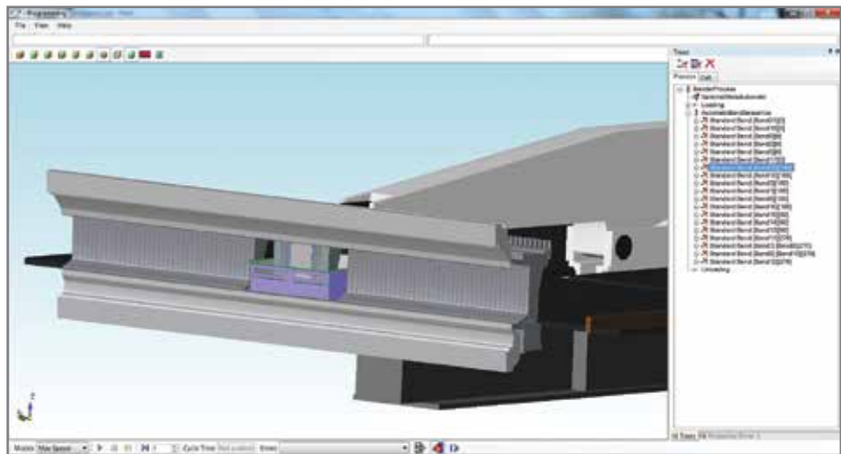
Part displayed and checked in 3D environment within MasterBend CAM
