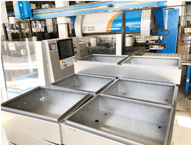
*The Prima Power EBe provides the high bending quality required in demanding applications. The quality is achieved through precise control of bending axes, fast and smooth bending motion, programming, and rigid construction.*
