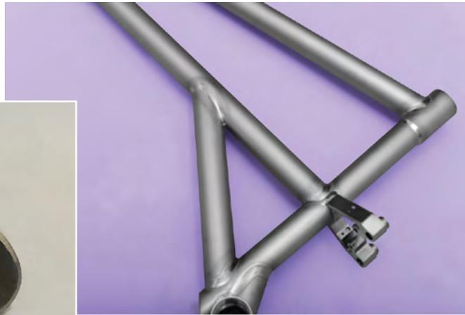
*Helix bike components are bevel-cut at many different steep angles on the LASERDYNE 430 BeamDirector® fiber laser system. All tubular components are made of high strength, light weight titanium. The bevel-cut process provides an edge finish that allows the parts pictured to mate perfectly without deburring prior to automated welding.*
