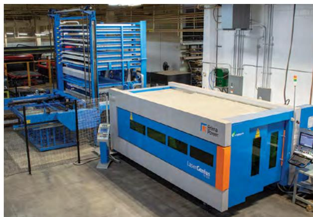
High-dynamic linear motors ensure a 15% increase in productivity compared with conventional drive systems. The Laser Genius has a comprehensive range of automation modules and the effective CNC proprietary management guarantees accuracy in cutting and head positioning.
