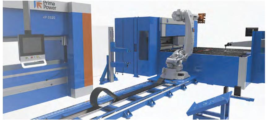
On the left: the eP-0520 press brake can operate with the robot or in manual mode.
