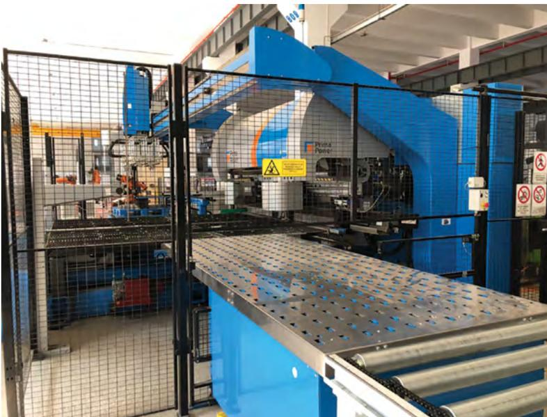
The EBe is available in models with a bending length of up to 149" (3,800 mm) and an opening height of 8" (204 mm).
