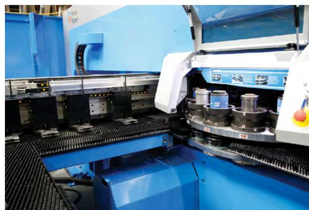
*A flexible turret concept with 16 rotating tool stations allows up to 384 tools or 128 rotating tools to be available in the turret at the same time.*
