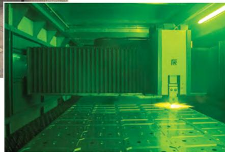
*The Prima Power fiber cutting head features single lens strategy, safe impact protection system, high dynamic focal axis with 35 mm stroke, lens drawer with quick alignment system (OPC), and protection glass drawer for easy inspection. These features make it an accurate, versatile, and efficient machine capable of 24/7 lights-out production.*
