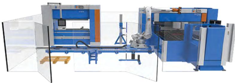
The system developed by Prima Power consists of a BCe Smart panel bender, an eP-0520 press brake, and an anthropomorphic robot mounted on a 7th axis.
