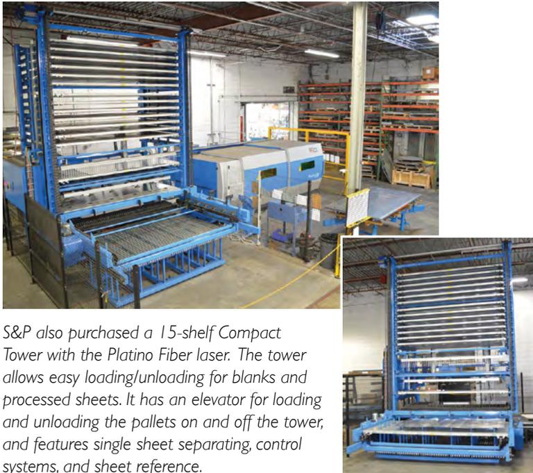
S&P also purchased a 15-shelf Compact Tower with the Platino Fiber laser. The tower allows easy loading/unloading for blanks and processed sheets. It has an elevator for loading and unloading the pallets on and off the tower, and features single sheet separating, control systems, and sheet reference.
