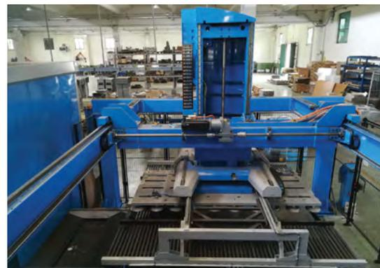
*The Prima Power Night Train FMS material management system supports C.M.C. in the quick changes of production, typical of orders with reduced and frequent batches.*
