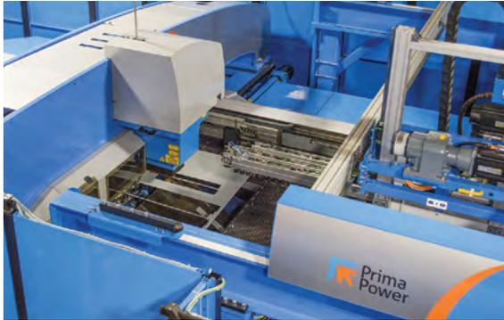
*The laser used in the system, as its most flexible tool, is a 4kW high-brilliance fiber laser. Cutting speed increases in proportion to power. A totally closed-cabin design for eye safety and noise reduction is always included with the system.*
