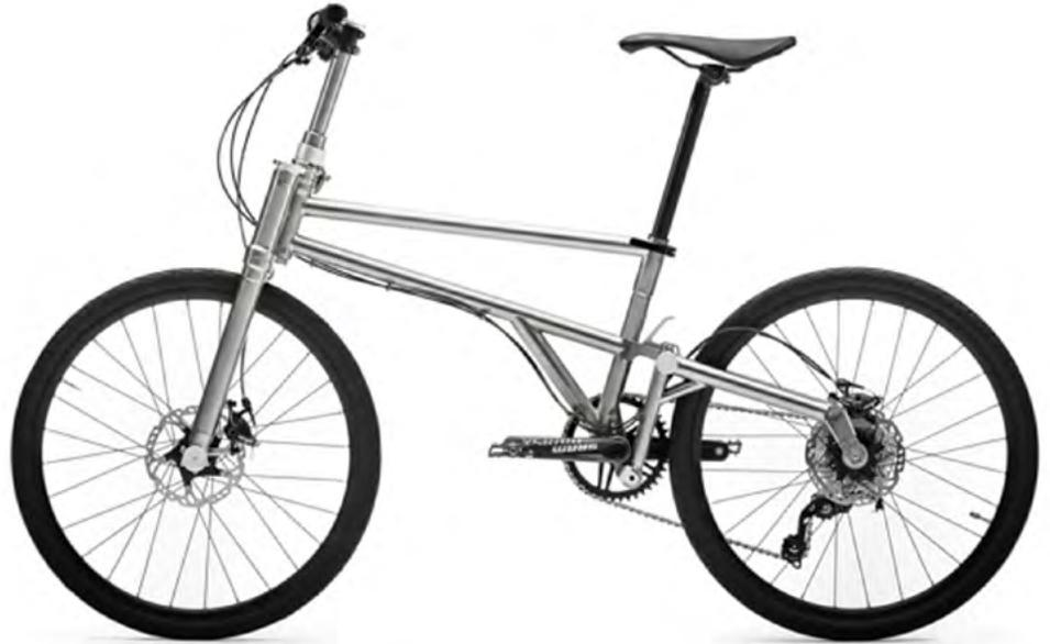
Claimed to be “the best folding bike on the planet,” the Helix bike side-by-side folding design puts the wheels beside the frame and between the cranks. The bike’s “go-anywhere compactness” with great performance and mobility, does it without sacrificing durability.
