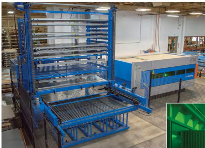
*The Compact TowerServer allows easy loading/unloading for blanks and processed sheets for lights out operation.*
