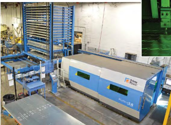
The Platino Fiber laser can be used to cut a wide range of materials. It cuts various thicknesses, up to 20 mm of mild steel, with efficiency and quality. Productivity increases particularly with thin and medium-gauge sheet metal.
