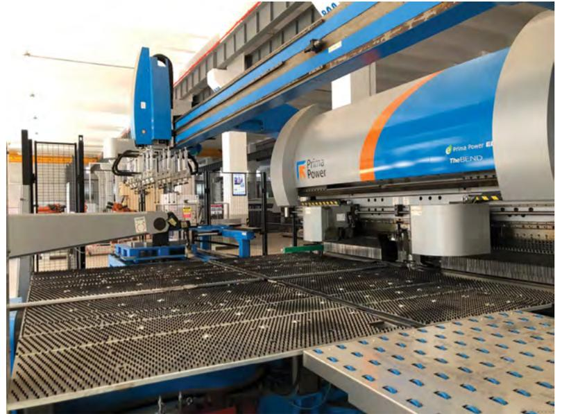
*The EBe servo-electric panel bender is a bending solution that is designed specifically for each fabricator’s production requirements to achieve maximum productivity, quality, and repeatability.*
