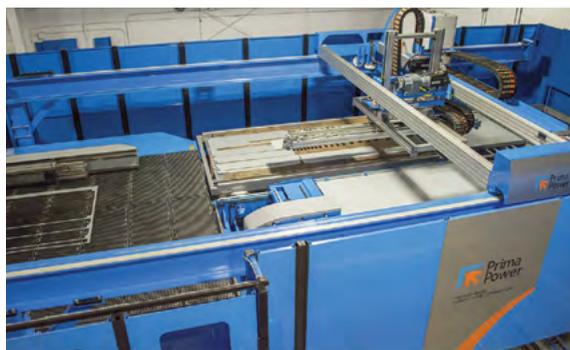
*P&A Metal Fab chose the high-performance portal type loading and stacking robot LSR to be integrated with its LPe6f. The LSR provides a reliable, fully-automatic process from loading to picking of parts and stacking them.*
