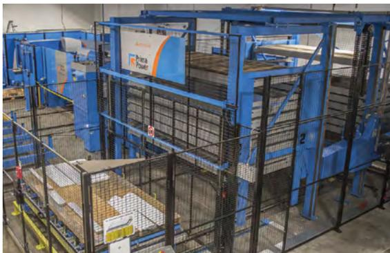
*Combo FMS Double-Sided Storage is a flexible material system with the compact COMBO storage as a key module in automating the material flow. It makes different materials available at the working point quickly and practically and can also serve as intermediate storage for ready components and as a buffer.*
