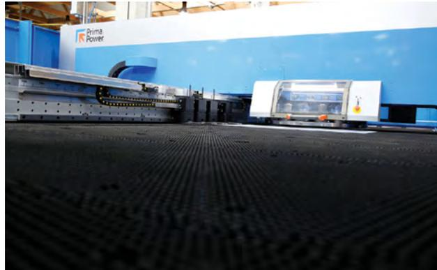
*The Combi Genius from Prima Power combines the advantages of servo-electric punching technology with state-of-the-art fiber laser cutting.*
