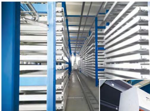
*The Prima Power Night Train FMS material management system allows C.M.C. greater efficiency in managing materials and processes.*
