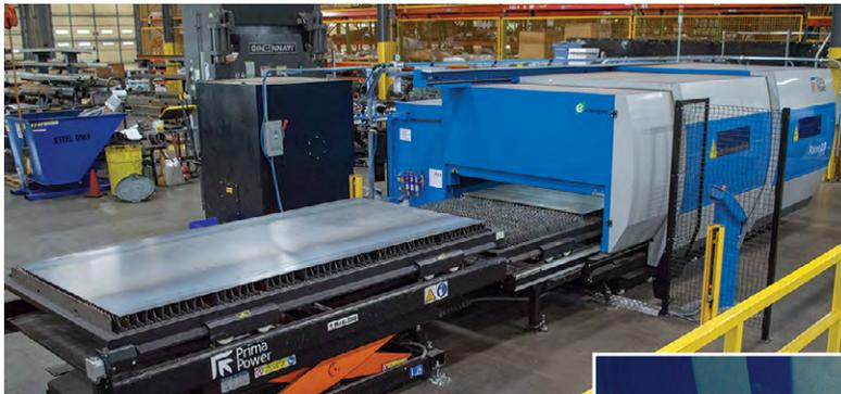
The Platino Fiber Laser has a single focusing lens system with an automatic nozzle changer. According to Finley, from a quality and productivity standpoint, the automatic nozzle changer eliminates the possibility of someone forgetting to change a nozzle or putting on the wrong nozzle.
