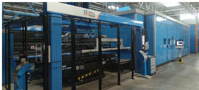
The Night Train system installed at Tehnos includes two Platino Fiber 1530 and a Combi Genius 1530, all equipped with LST sorting systems. A robotic bending cell is also being integrated.
