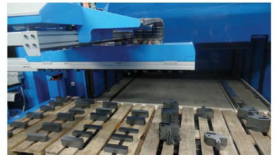
Prima Power's LST sorting system is able to palletize even pieces with complex geometries, thus allowing a fully automated production flow.
