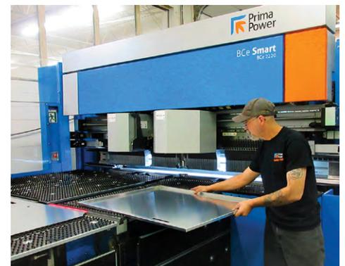
The BCe Smart with its innovative servo-electric bending technology is the optimal solution for medium production volumes as well as for low volume or lean production. It guarantees precision and repeatability with a considerable reduction of maintenance costs.
