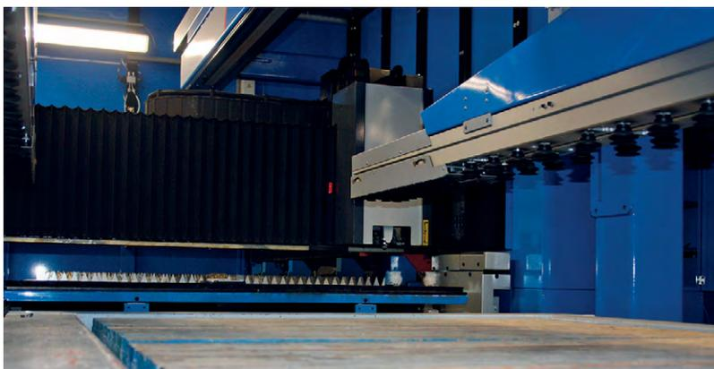
The Night Train also integrates Prima Power Laser Genius 1530, a 2D fiber laser cutting system equipped with a 6kW fiber source and an automatic stacking robot for LST laser machines.
