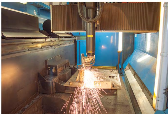
The Laser Next 1530 is primarily used for the hot stamping part of the company's business including R&D work, prototype work, production tool tryout, and process development including laser cutting development, and low-volume production.
