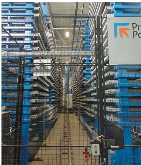
*The Night Train Flexible Manufacturing System allows optimal management of raw materials, semi-finished products and scraps, allowing a single operator to control all production.*
