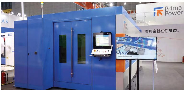
The second product was the Combi Sharp, a combination laser/punch machine with high energy efficiency, low maintenance requirements, and fast operation speed. The Combi Sharp combines superior laser cutting with the ability to do forming, tapping, and marking.
