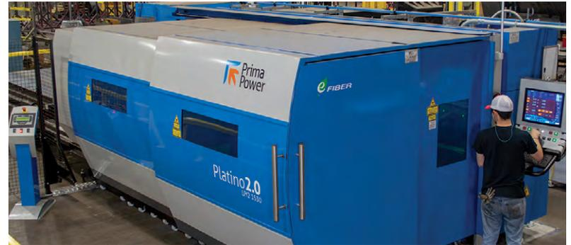
Prior to acquiring the Prima Power laser, UE Manufacturing used to outsource a majority of its sheet metal fabrication. The company purchased the Platino 6kW Fiber Laser in 2018 to alleviate its dependence on outsourcing.
