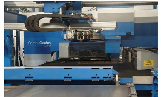
*The 4 kW fiber source and the punching unit with over 300 tools allow the Combi Genius to process sheet metal up to 8 mm.*
