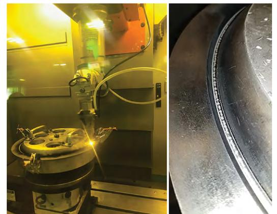
*Two part Hastalloy® X assembly pictured left during the automated welding process. The new LASERDYNE 430 system precisely controls the power, position, and focus for a perfect end result without cracks or voids in the weld structure.*
