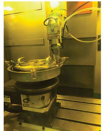
*Prima Power Laserdyne's BeamDirector assembly contains the weld head with integrated air knife. Lens protection is ensured with the air knife function for cooling the lens and deflecting weld debris.*
