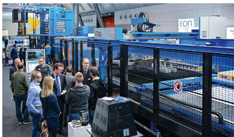
In Stuttgart, Prima Power also displayed the high-performance **Laser Genius 1530** fiber laser machine with 10kW laser, featuring new cutting strategies allowing top performance of cutting speed, piercing time, and reduction of gas consumption. The machine was showcased with the Combo Tower Laser, a flexible storage system integrating loading and unloading for the optimal solution in lights-out production.
