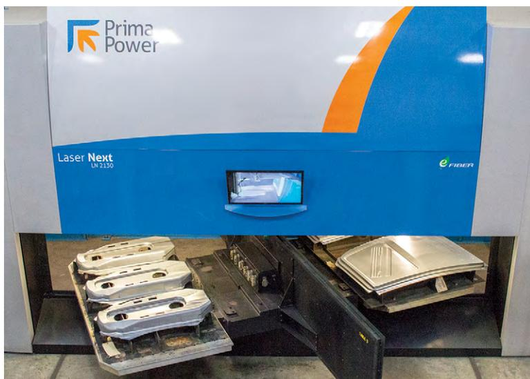
*The Laser Next's high accuracy, repeatability, and precision have allowed Diversified to replace some dies and pierced dies with laser cutting, making the process more competitive for its customers.*
