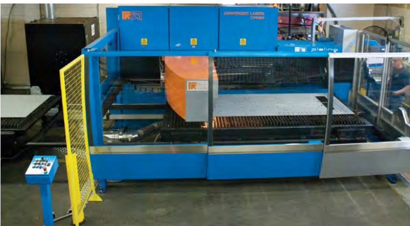
Offering a compact footprint along with a Cartesian Cantilever structure that provides three-sided access, Platino is a cost-effective machine that is easy to operate and quick to program.
