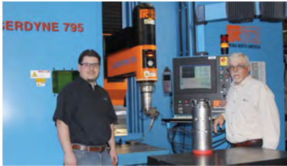
Shown with a recently purchased Laserdyne 795 BeamDirector systems are (left to right) Kurt Magedanz, Process Engineer and Ed Magedanz, Senior Manufacturing Engineer of Ace Precision Machining Corporation. The systems are used for processing complex aerospace components similar to the one pictured on the worktable.
