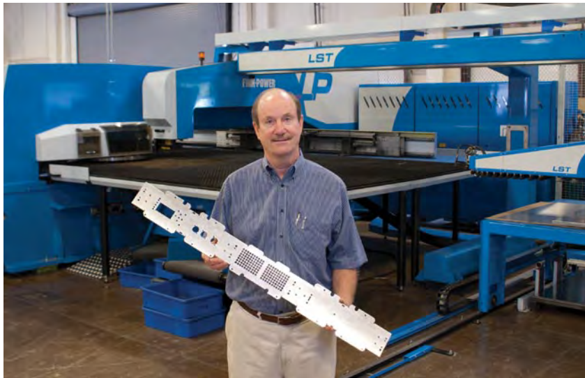
C.A. Theis chose the Prima Power LP6 laser/punch combination with the LST6 load and stacking robot.
