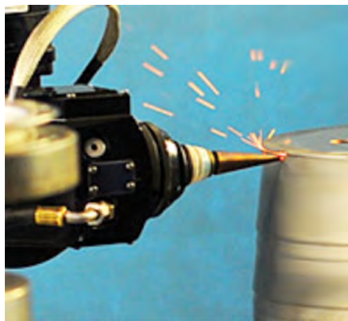
One of five Co2 laser systems ranging from 1700 to 4000 Watts used for cutting, trimming, welding, and hole drilling.
