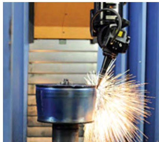
With nine Laserdyne multi-axis laser systems in-house, Ace Precision is equipped and experienced at the most complex projects requiring laser processing. As pictured, these include drilling effusion cooling holes in very dense patterns at shallow angles holding hole diameter tolerances of less than 0.002 inch.
