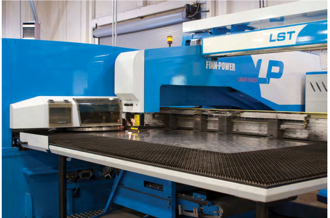
Optimum use of the Prima Power LP6 means that a fabricator can use the turret punch press where it is easier or faster, and the laser where it is the most effective.
