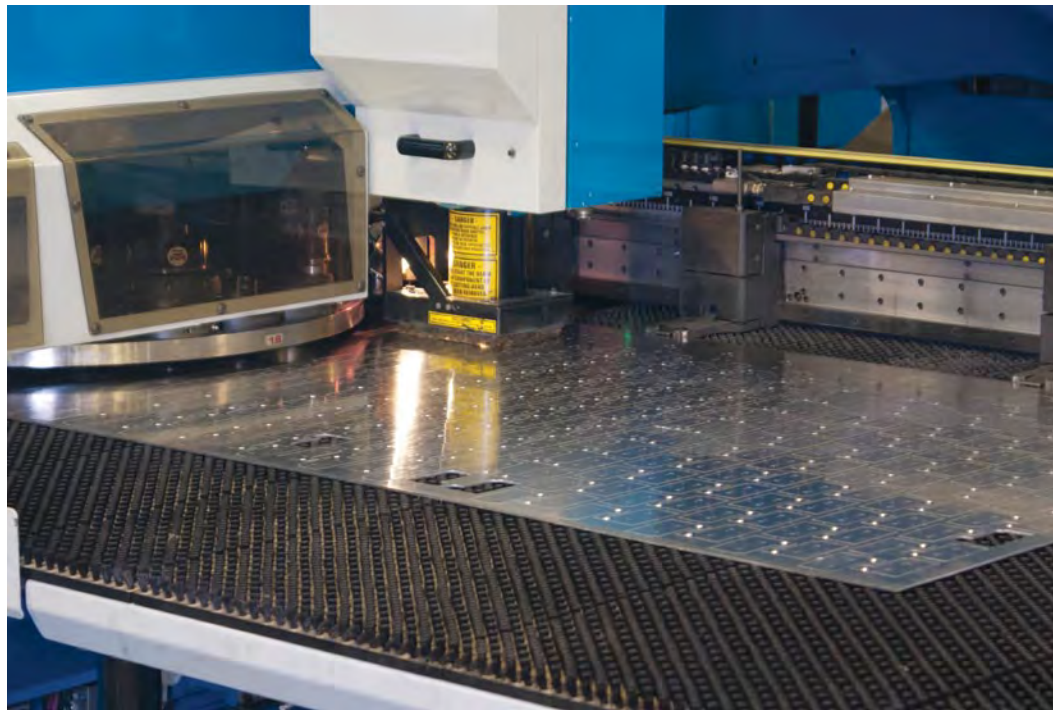
The Prima Power LP combines the unique C-Series 20-station turret punch press with the latest generation of CO2 lasers.
