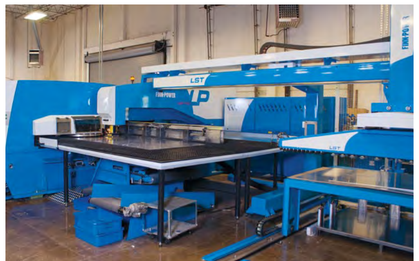
The LP6 has the ability to utilize full sheets while eliminating the need to shear to size blanks being processed.
