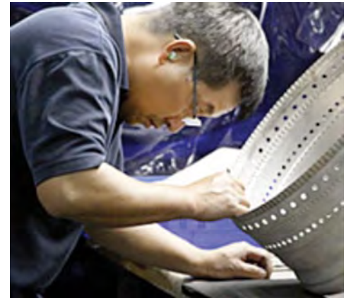
Ace Precision manufactures engine components for the commercial and defense industries. A laser-processed engine component is pictured being visually inspected. Ace Precision has experience with many engine designs including military platforms for Apache and Chinook helicopters, Abrams M1 Battle Tanks and B2, F18, F22 and F35 aircraft.
