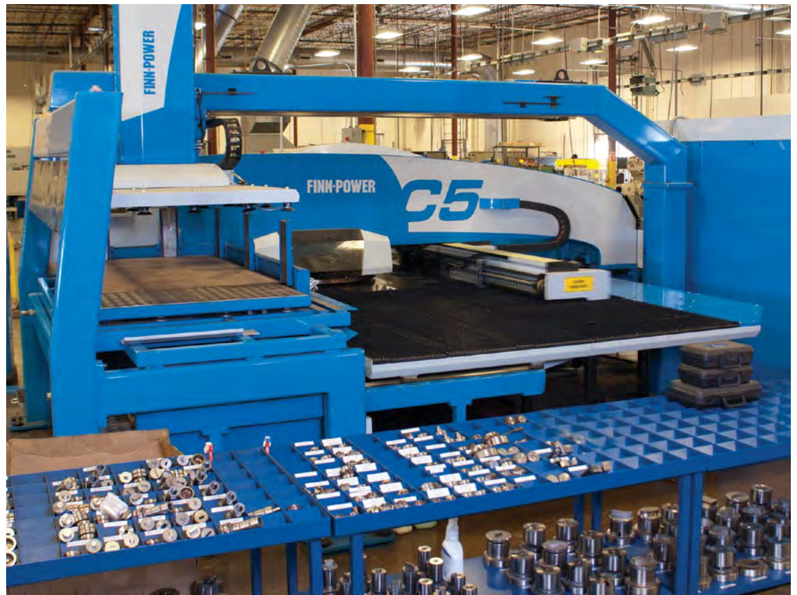
The C5 Express adds unmanned operation to the C5 turret punch press through highly compact load/unload automation. The unit's loading/unloading solution utilizes the space above and below the machine, requiring only slightly more space than a turret punch press.
