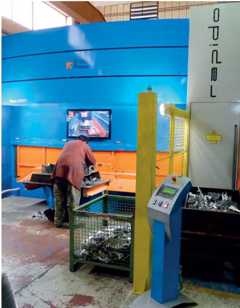
The turntable allows workpiece loading and unloading in total safety, while the machine is operating.
