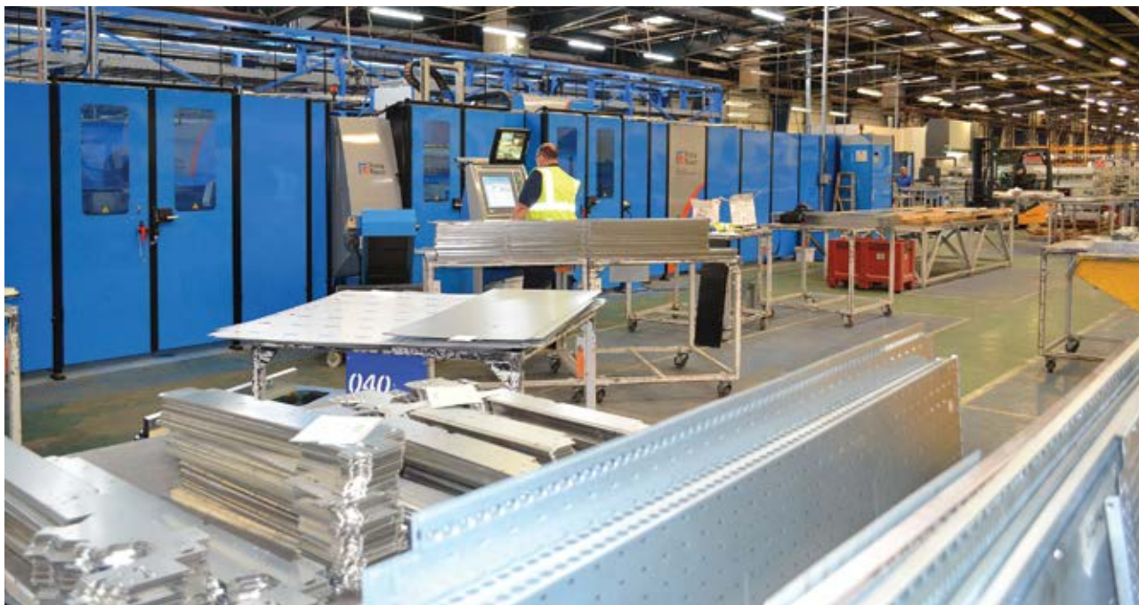
The Night Train FMS is able to perform high-speed laser cutting, punching and forming, as well as the storing of raw and processed material and parts. Prima Power's LPe8f Combi machine lies at the heart of the highly productive FMS that was designed to satisfy Epta UK's specific demands.
