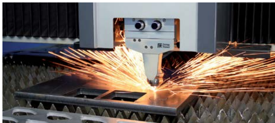
The Platino Evo is equipped with a new cutting head with adaptive collimator designed and manufactured by Prima Power. It is a fiber laser cutting head with adaptive optics for automatic management of the focus position and focus radius diameter.
