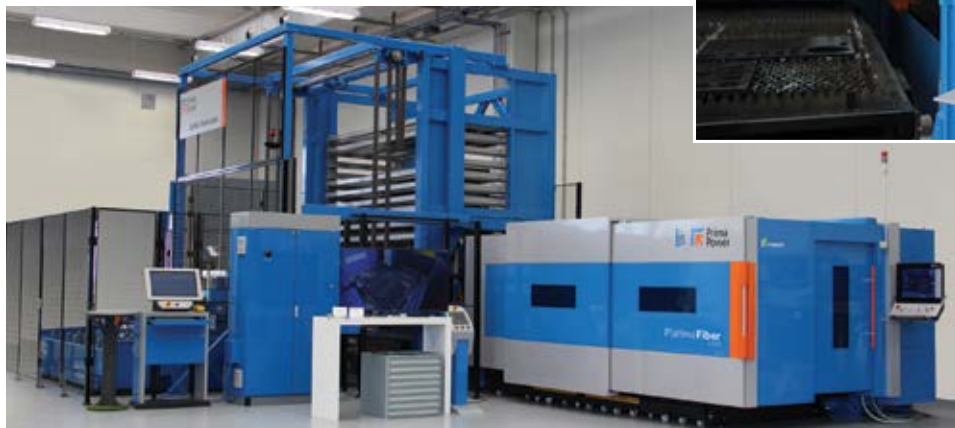
The Platino Fiber Evo features the latest generation numeric control designed and manufactured by Prima Electro. Its main functions include laser parameters monitoring and management, work programs editing, and programming management with a complete preview function.
