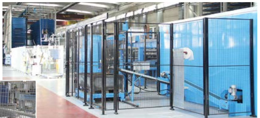
The first unit of the line consists of the SBe6 punching-shearing machine. It is a completely servo-electric machine with sheet handling performed using linear motors that increase the speed of placement up to 210 m/min (part of the machine structure is made of composite material), greatly increasing productivity.
