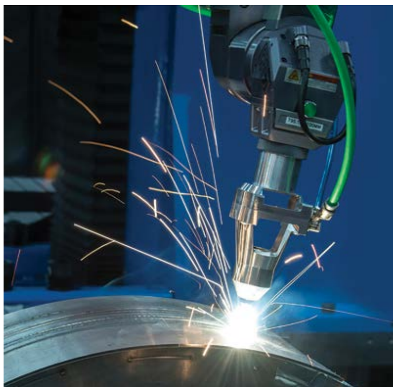
Photo Three: SmartShield™ patent pending nozzle assembly protects the lens coverslide using clean compressed air while supplying shield gas, such as nitrogen or argon, to protect the weld from oxidation.
