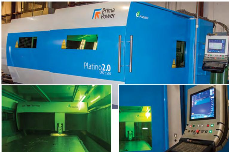
The Platino Fiber cuts various thicknesses, up to 20 mm of mild steel, with efficiency and quality. Numerical control, operator interface, and programming software are user-friendly and smart tools, which are developed and manufactured by Prima Power.
