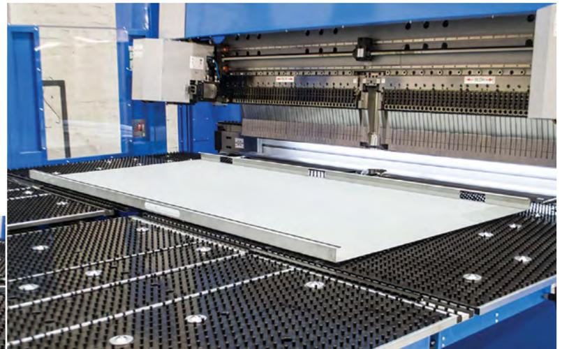
*The BCe Smart has a highly robust and stable design consisting of a static machine frame on which a moving C frame is mounted to hold and control the bending blades. A versatile upper tooling system is utilized for clamping while a manipulator arm automatically rotates and positions the part for every bend. A brush-top loading and unloading table provides both optimum support and scratch-free material movement.*
