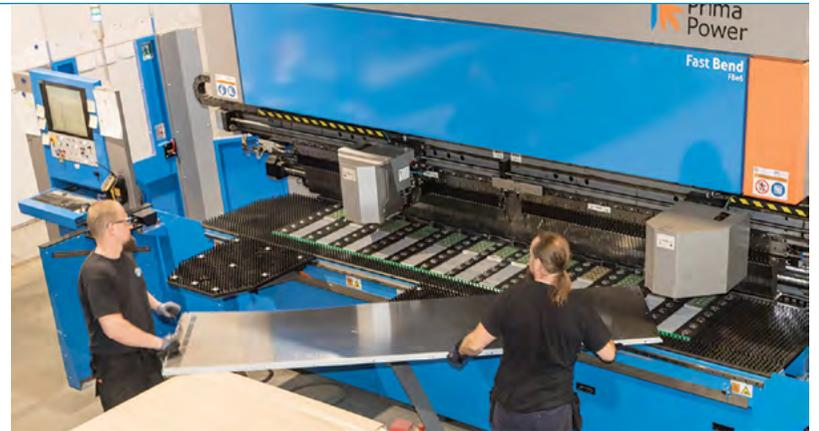
The semi-automatic FastBend panel bender is an essential part in the production of facade panels.
