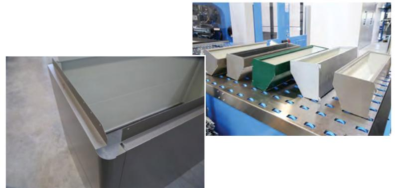
For the production of parts such as this body (left) or the new Floraboard (right), the new bending machine requires less than a third of the time needed by conventional press brakes to do the same job.
