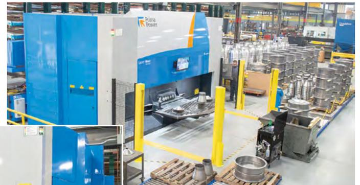
*The linear motors on the main axes and the direct drives on the laser head, combined with advanced control systems – guarantee the highest performance, consistently with the utmost precision.*
