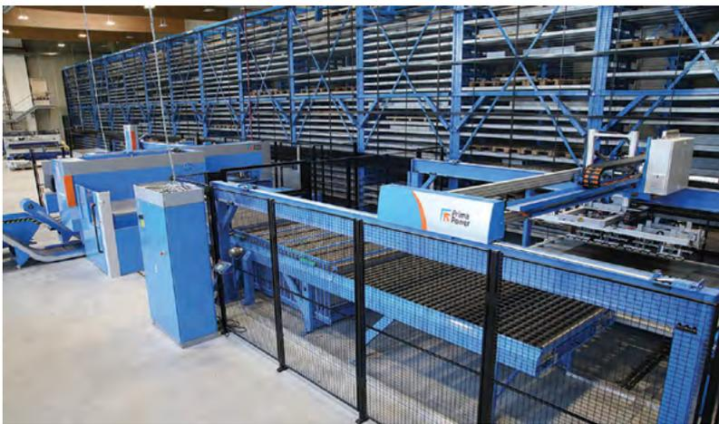
50-meter long Night Train Brilliance has 560 storage box locations (each with a four-ton capacity) to store raw materials and finished stamping blanks. The PSR gripping and stacking robot (right) automates the return of punched plate blanks into the sheet metal warehouse.
