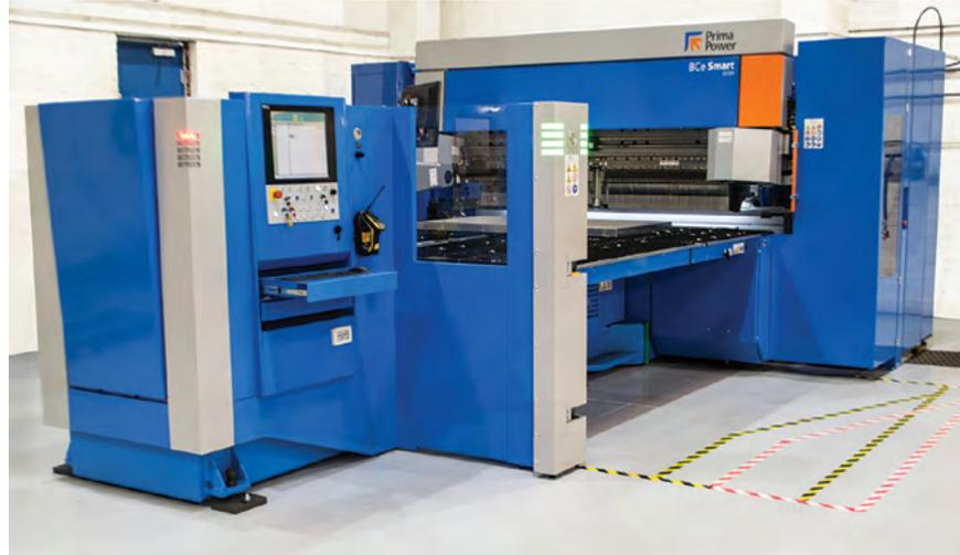
*The Prima Power BCe Smart 2220 has a maximum bending length of 2,250 mm and height up to 204 mm and is able to automatically position, bend, and manipulate sheet metal parts for a fully-automatic bending process.*
