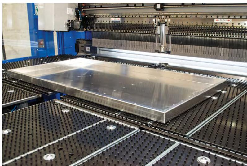
*A wide variety of bend profiles are fully achievable with the BCe Smart, including conventional single bends, compound and re-entered bends, flattening, and radial forming in materials up to 3 mm in mild steel, 2 mm in stainless steel, and 4 mm in aluminum.*
