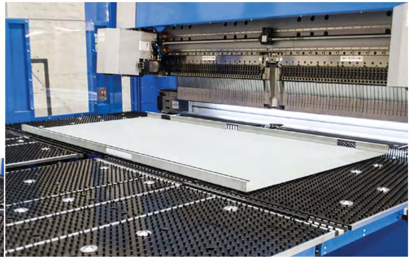
*The BCe Smart has a highly robust and stable design consisting of a static machine frame on which a moving C frame is mounted to hold and control the bending blades. A versatile upper tooling system is utilized for clamping while a manipulator arm automatically rotates and positions the part for every bend. A brush-top loading and unloading table provides both optimum support and scratch-free material movement.*
