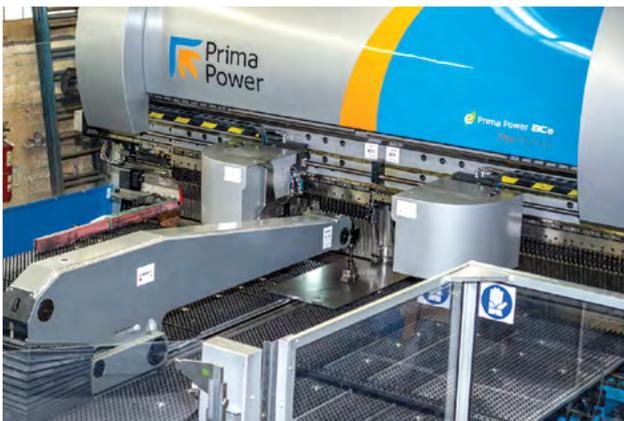
*The operation of the BCe is semi-automatic. It is a productive solution for small batches as well as for serial manufacturing. Total manufacturing time is shortened as the loading operation is simultaneous with the unloading of the ready-bent component.*
