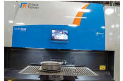
*When you're opening the door and loading a part, the laser isn't running parts. Kryton was looking for a machine that could load a part while it was running a part. The company chose the Prima Power Laser Next.*
