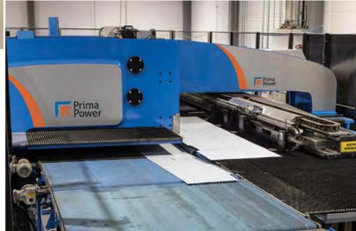
The biggest leap in PRP's production development was made in 2017, when the company invested in a Prima Power Shear Brilliance punching/right angle shearing unit with STS stacking automation.
