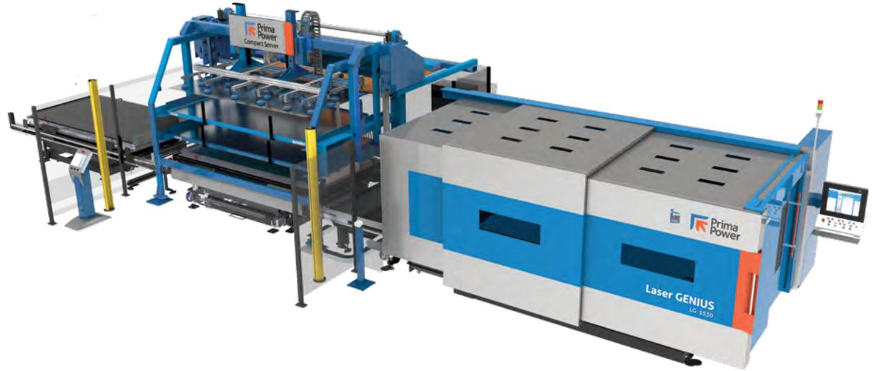
and stacking. The Prima Power line for the automated sheet metal flow, including Compact Server, Combo Tower Laser, LST, and the connection to the Night Train FMS, makes the machine an ideal system for continuous 24/7 production of two-dimensional pieces for every production requirement.
