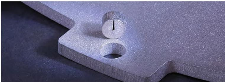
*Intricate features with precise positioning and dimensions are possible using the SmartPierce™ laser process.*
