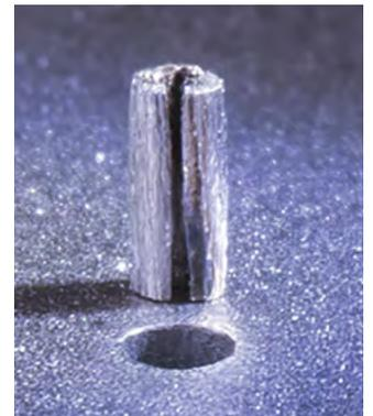
*SmartPierce is equally effective for thick or thin metals with a debris-free, clean pierce. Pictured behind the laser trepanned hole is the slug from the hole. The clean, narrow pierce leads to a well-controlled, high-quality hole with negligible debris.*
