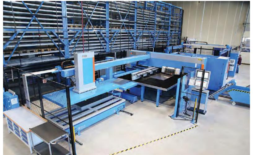
To punch the required parts, the Shear Genius punch-shear combination system by Prima Power was chosen. Connecting another punching machine would still be possible. (Pictures: x-technik)
