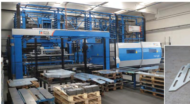
The introduction of this fully-automated laser cutting system makes it possible for Depedri to offer great cutting quality for steel, stainless steel, aluminum, copper and brass.
