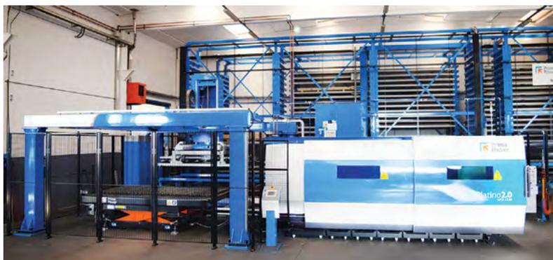
The Platino Fiber 2.0 laser machine's productivity is further enhanced by the combination with a Prima Power Night Train FMS warehouse, to manage the sheet metal to be loaded as well as handling the finished parts, which makes it an extremely efficient system.
