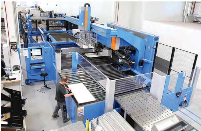
The fully-automatic Prima Power bending machine, the EBe 5.3, is supplied with punched plate blanks from the Night Train via the PSR picking and stacking robot for optimal production flow.
