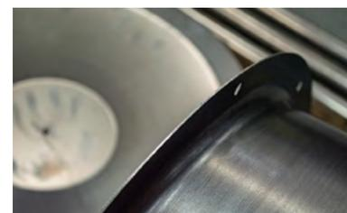
*Kryton management believes that the Laser Next cut quality is the best they have seen. The company now cuts aluminum by using high-pressure air cutting... and there is no burr. Kryton no longer has to do any secondary deburring operations.*
