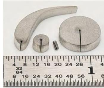
Photo shows slugs from precision cutouts of airfoil shapes and round holes in 3.5 mm thick stainless steel. The clean, high quality start is made possible by the LASERDYNE SmartPierce™ process.
