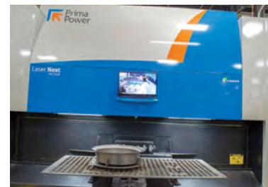
*When you're opening the door and loading a part, the laser isn't running parts. Kryton was looking for a machine that could load a part while it was running a part. The company chose the Prima Power Laser Next.*
