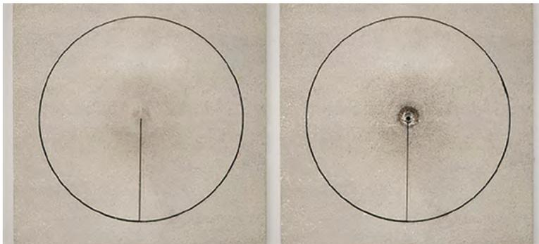
Laser cuts in 10 mm thick 304 stainless steel. The pierce point with SmartPierce (left) is the same diameter as the cut width (kerf). Using a traditional piercing method with fixed laser parameters (right), the pierce diameter is much greater compared to that using the SmartPierce process.
