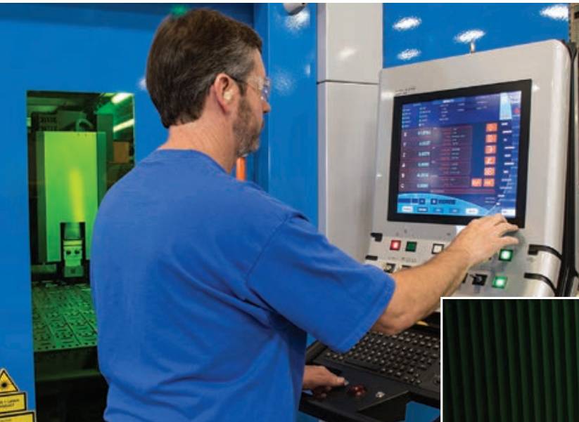
Linear motors provide enhanced speed up to 240 m/min. And the user-friendly proprietary CNC features a 17" LCD touch screen and trackball.
