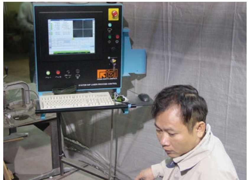
Using LASERDYNE'S through-the-lens viewing system (45 times actual size), the system operator positions the laser nozzle and enters the command for recreating each hole.
