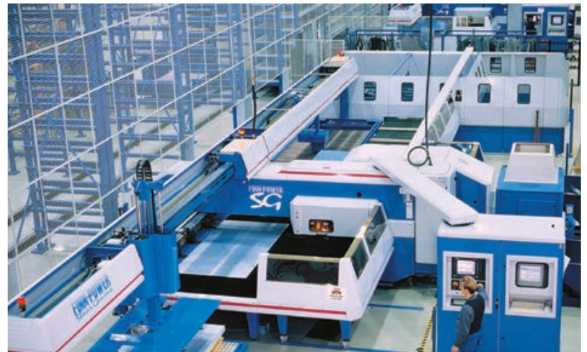
Shear Genius in 1998 with loading, unloading, and stacking automation.
