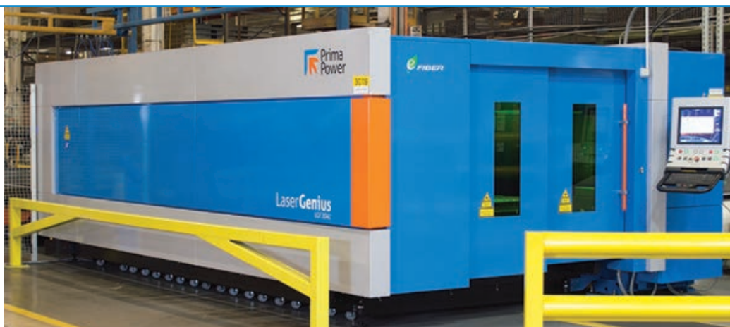
Laser Genius is the high-range 2D laser cutting machine, designed for very high productivity, quality, and flexibility. Its main features include linear motors and the innovative application of synthetic granite and carbon fiber. The Laser Genius features the smallest footprint on the market today.
