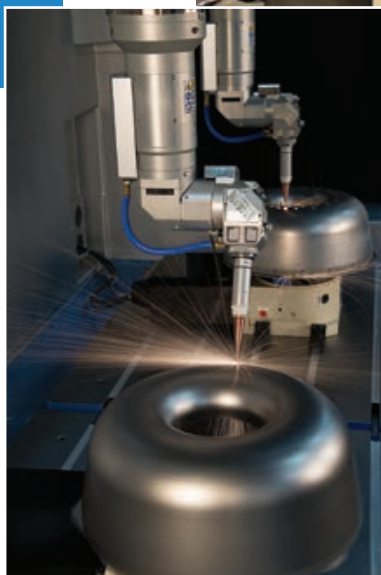
LASERDYNE BeamDirector® technology is included in both 606D workstations. It allows drilling at angles as shallow as 10 degrees from the surface throughout the entire work envelope.
