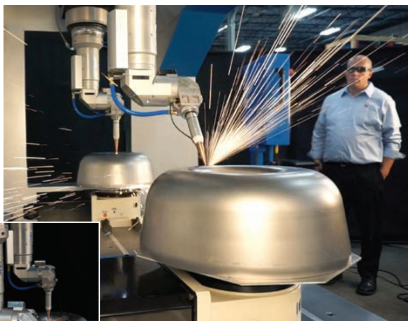
The 606D is shown percussion drilling (foreground) cooling holes in an aerospace engine combustor dome assembly while simultaneously cutting larger holes in a similar aerospace component on the second workstation (background).
