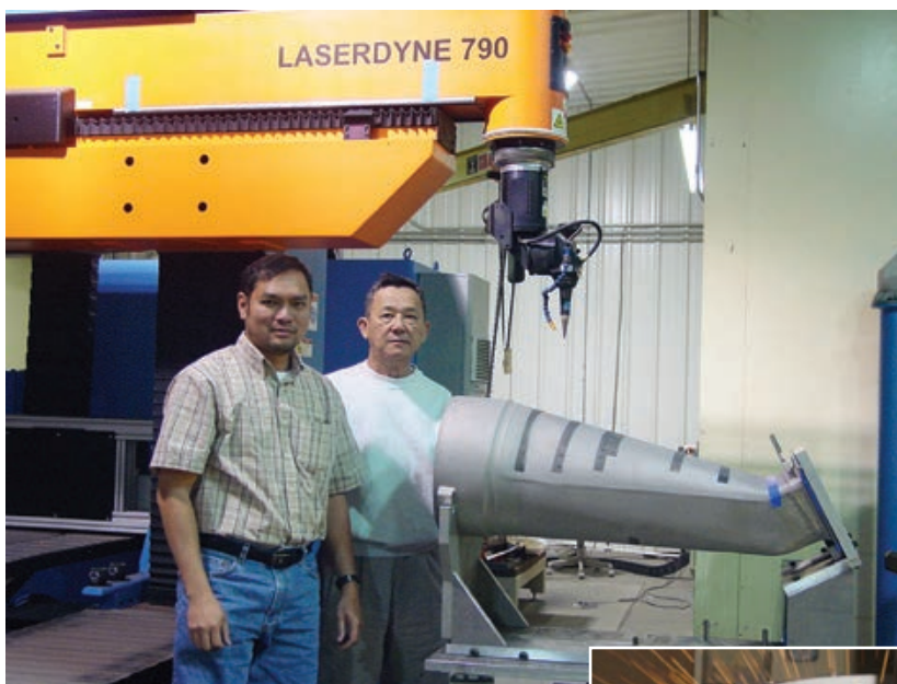
Quang Tran, president (right) and Son Dao, operations manager of TL Precision Welding, Inc., stand adjacent to a refurbished gas turbine component laser processed with the company's LASERDYNE 790 BeamDirector system.
