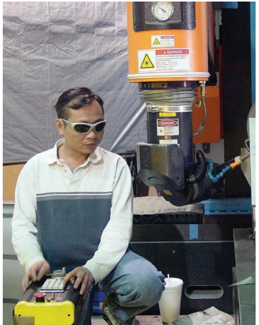
Operator is shown programming the Optical Focus Control (OFC) feature of the LASERDYNE Beam Director system.
