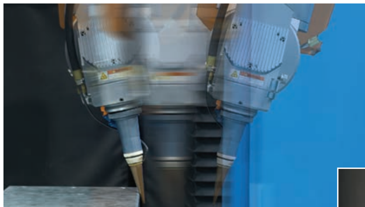
LASERDYNE BeamDirector® technology is included in both 606D workstations. It allows drilling at angles as shallow as 10 degrees from the surface throughout the entire work envelope.
