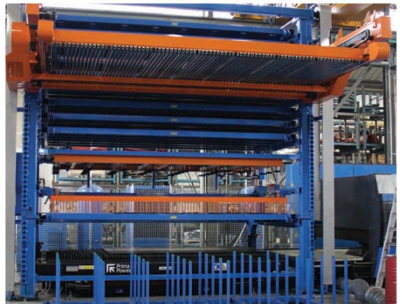
Detail of 10-pallet automation tower at the service of the Prima Power Platino laser cutting machine.
