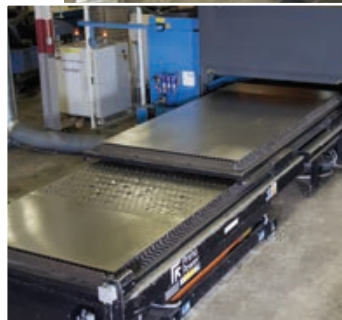
The Platino Fiber Laser cuts various thicknesses, up to 20 mm of mild steel, with efficiency and quality. Productivity increases particularly with thin and medium-gauge sheet metal.
