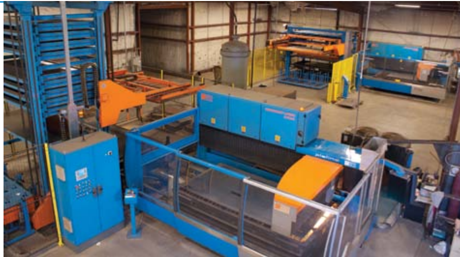
The Prima Power Platino is equipped with lasers developed and produced at Prima Electro in laser powers ranging from 3000 to 5000W. The laser cuts a broad range of materials and thicknesses with speed and precision without the need for manual adjustments.
