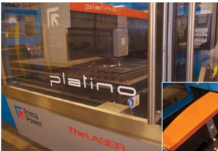
Platino’s laser cutting head gives users a choice of a 10-inch focal length in addition to the standard 5-inch and 7.5-inch lenses. The 10-inch lens enhances the application flexibility by increasing the depth of focus and enlarging the spot diameter for high and uniform cut quality of thick stainless (5/8 in), thick aluminum (1/2 in) and thick mild steel (1 in).
