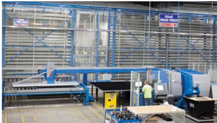
The centerpiece of the Finn-Power automated sheet processing system is the Night Train Material Management System, which is the inventory and material transporting center.
