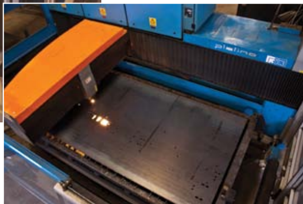
Platino’s laser cutting head gives users a choice of a 10-inch focal length in addition to the standard 5-inch and 7.5-inch lenses. The 10-inch lens enhances the application flexibility by increasing the depth of focus and enlarging the spot diameter for high and uniform cut quality of thick stainless (5/8 in), thick aluminum (1/2 in) and thick mild steel (1 in).
