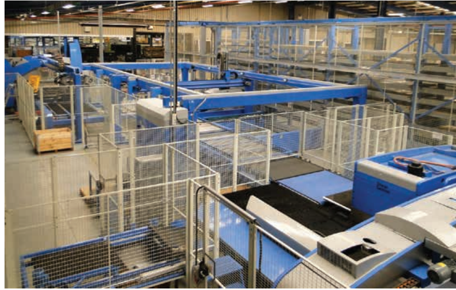
Caption goes here. Once the flat part comes off the Shear Genius SGe5, it is picked up by a robot, which automatically alters the position of the lifting suckers to avoid apertures and to fit the component shape.
