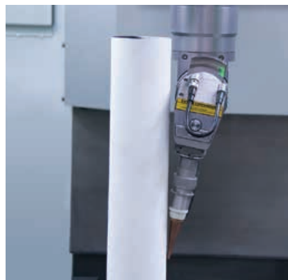
High speed drilling on turbine engine components using the LASERDYNE 795XL. It has exclusive OFC (Optical Focus Control), BTD (Breakthrough Detection) and CylPerf programming at shallow and compound angles. This fiber laser system meets every challenge for producing cooling holes in today's increasingly complex aerospace engines.
