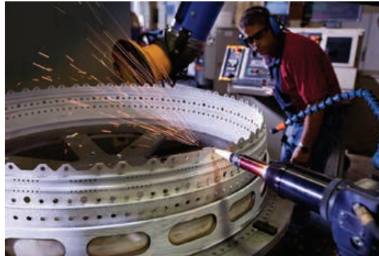
Gary Loring, laser supervisor/engineer for Paradigm Precision with PRIMA POWER LASERDYNE's newest laser addition—a remanufactured LASERDYNE 890 BeamDirector system equipped with a fiber laser. The system is used to produce complex cooling holes in turbine engine components.
