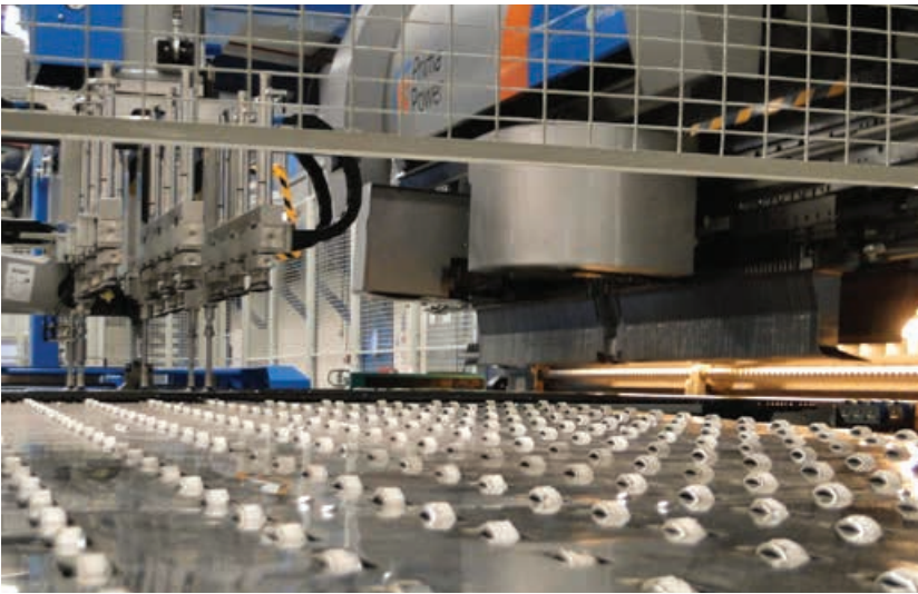
The bending machine is robot loaded, and automated tool changing makes changing from one series of bending sequences to another, as each different component arrives, something that takes just a few seconds.
