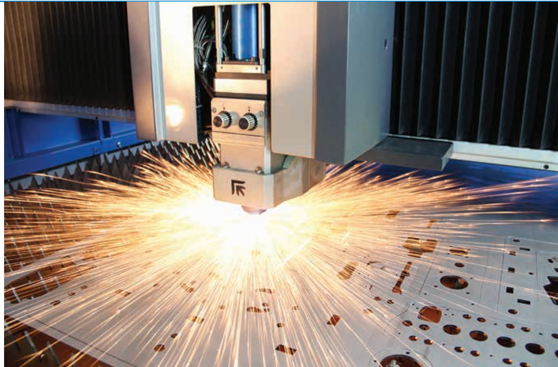
The Prima Power fiber laser cutting head features single lens strategy, safe impact protection system, high dynamic focal axis with 35 mm stroke, lens drawer with quick alignment system (OPC), and protection glass drawer for easy inspection. These features make it an accurate, versatile, and efficient machine capable of 24/7 lights-out production.
