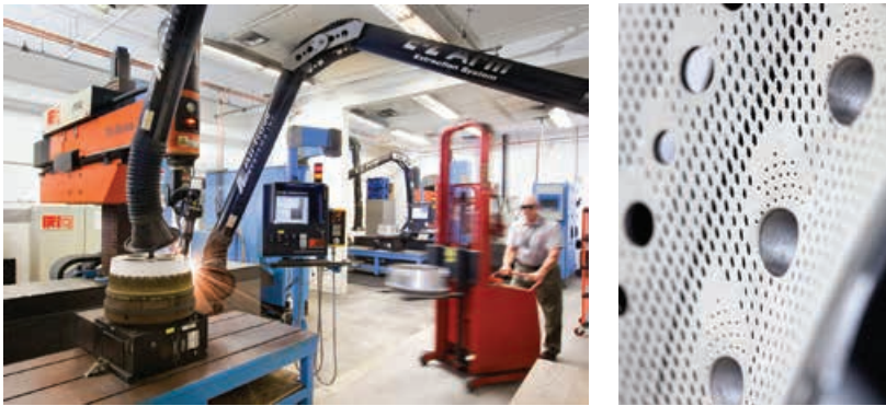
A LASERDYNE 795 XL system shown processing a turbine engine component with thermal barrier coating.
