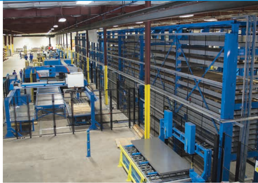
The centerpiece of the Prima Power automated sheet processing system is the Night Train Material Management System, which is the inventory and material transporting center.
