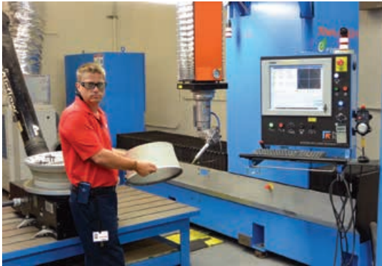
Gary Loring, laser supervisor/engineer for Paradigm Precision with PRIMA POWER LASERDYNE's newest laser addition—a remanufactured LASERDYNE 890 BeamDirector system equipped with a fiber laser. The system is used to produce complex cooling holes in turbine engine components.
