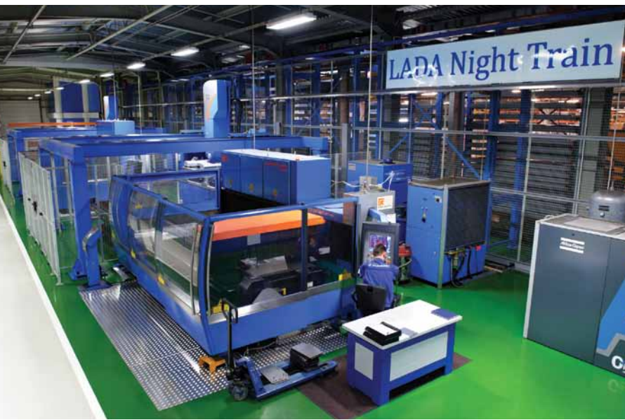
LADA-FLAKT's Night Train FMS line includes two laser machines, two punch/laser combination machines, five auxiliary robots, an automatic bending center EBe5, and three loading/unloading modules.
