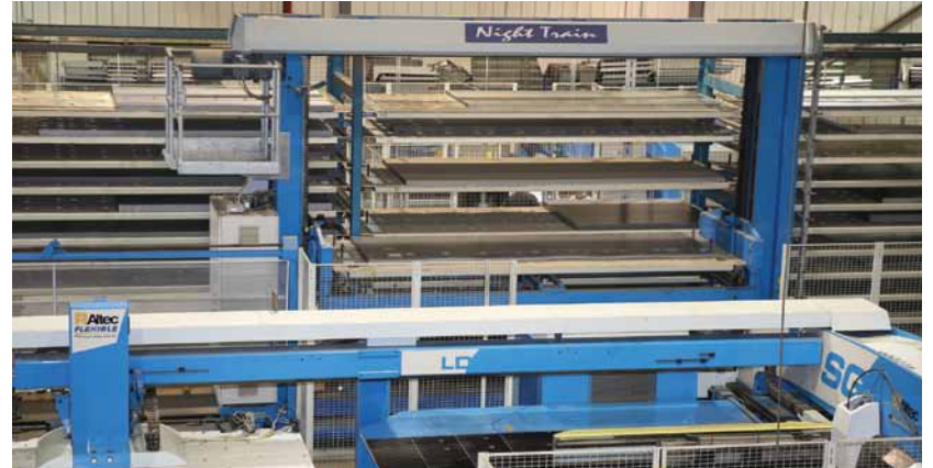
The centerpiece of the Prima Power automated sheet processing system is the Night Train Material Management System, which is the raw material inventory and work-in-process staging center.
