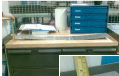
Bowed parts after punching and shearing and laser cutting.
