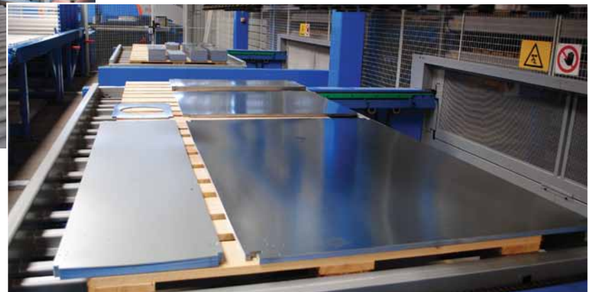
The bending operation is fully automated, from the loading of flat punched parts to unloading of the finished product.
