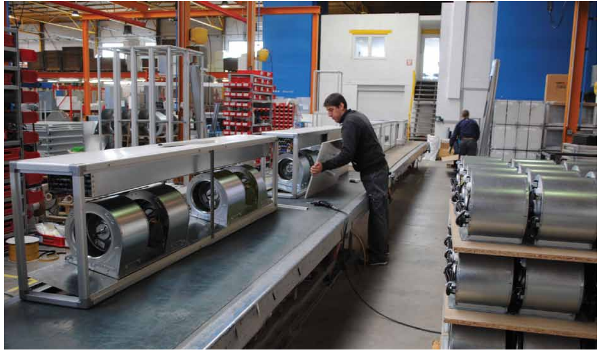
Assembly of small ventilation boxes.
