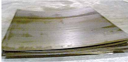
Bowed material that is not stress relieved.
