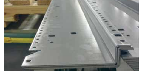
Under-bent parts due to material quality issues (excessive tensile strength and hardness)
