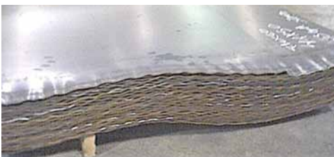
Example of poor-quality, rolled, levelled, and straightened material.
