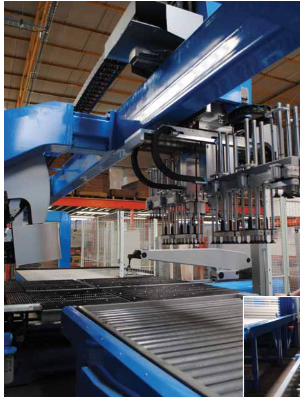
The bending operation is fully automated, from the loading of flat punched parts to unloading of the finished product.
