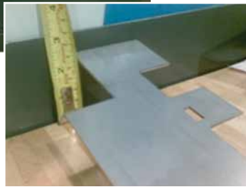
Bowed parts after punching and shearing and laser cutting.
