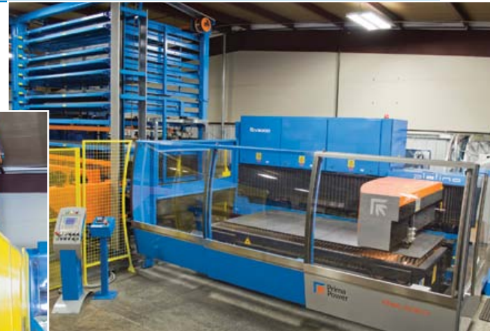
Prima Power's Compact 10-shelf TowerServer allows easy loading/unloading for blanks and processed sheets. It has an elevator for loading and unloading the pallets on and off the tower, and features single sheet separating, control systems, and sheet reference.
