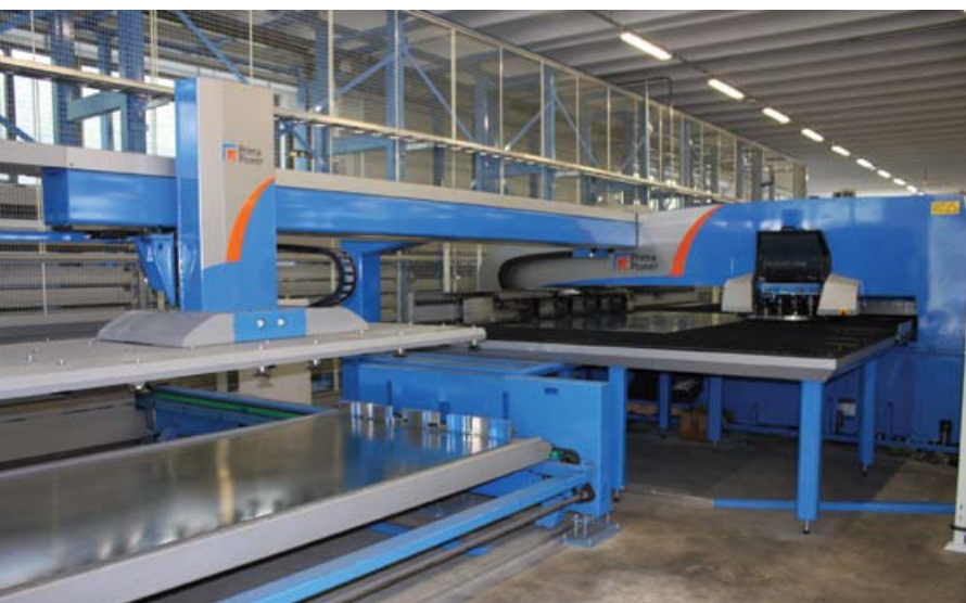
To meet the demands of its customers, C.L.A. invested in the Prima Power Shear Genius SGe6, integrated punching and shearing machine.
