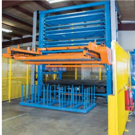
Prima Power's Compact 10-shelf TowerServer allows easy loading/unloading for blanks and processed sheets. It has an elevator for loading and unloading the pallets on and off the tower, and features single sheet separating, control systems, and sheet reference.
