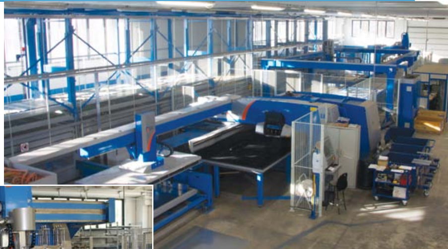
The EBe5 bending machine chosen by C.L.A. is able to perform the bending lengths up to 2,650 mm.
