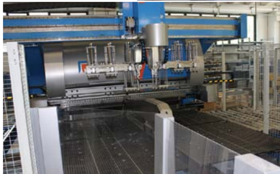
The EBe5 bending machine chosen by C.L.A. is able to perform the bending lengths up to 2,650 mm.
