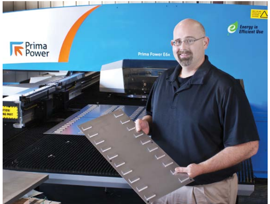
Jason Redmon, vice president, engineering, inspects a part fabricated on the Prima Power E6x servo-electric turret punch press.
