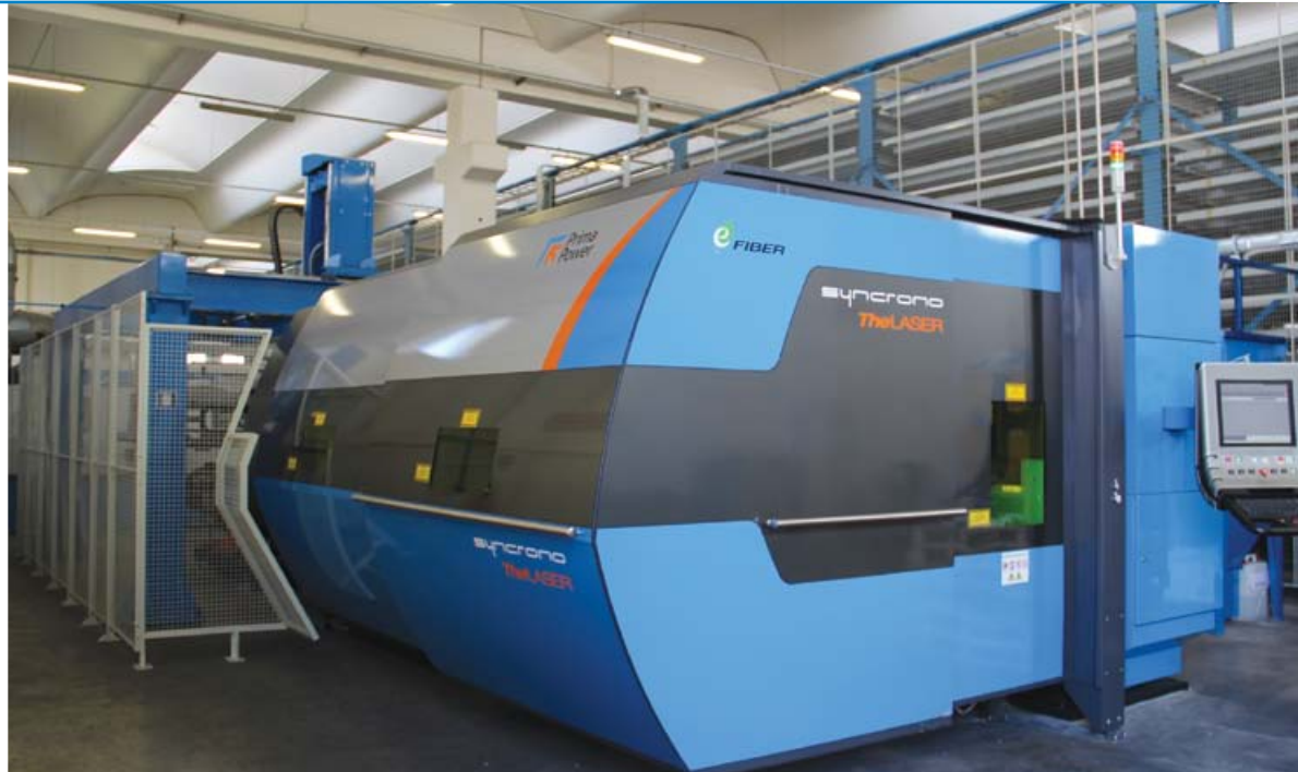
The Sincrono Fiber is a machine that has thin cuts in its DNA. Moreover, in the specific case of Rizzato, its 2 kW fiber source meets the need of having to cut complex parts, in which it is necessary to make very rapid movements and changes of direction in short strokes.
