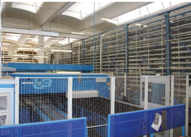
The Sincrono Fiber is a machine that has thin cuts in its DNA. Moreover, in the specific case of Rizzato, its 2 kW fiber source meets the need of having to cut complex parts, in which it is necessary to make very rapid movements and changes of direction in short strokes.
