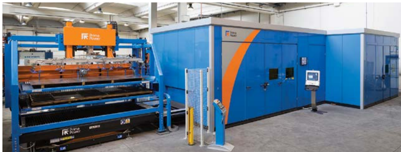
System with Platino Fiber and Compact Server for handling sheets.
