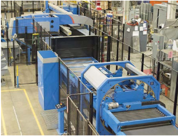
The Prima Power PSBB is a compact, flexible manufacturing line that processes blank sheets into high-quality components that exit fully bent.
