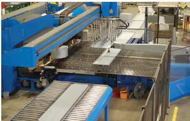
The EBe servo electric Express Bender is a bending solution that is designed specifically for each fabricator's production requirements to achieve maximum productivity, quality, and repeatability. The bending operation is fully automated, from the loading of flat punched parts to unloading of the finished product.
