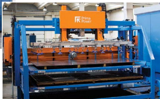
Compact Server for loading and unloading blanks and processed sheets.
