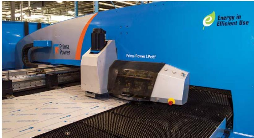
The high-end premium series turret punch press of the LPe6f has properties such as automatic tool length measurement, optimization of stroke length and easy adjustment of the punching stroke. These combine with others, adding up to faster set-ups and more ease of operation.
