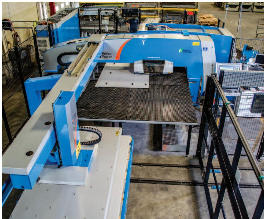
*Improved accuracy and repeatability from the punch-shear combination machine has led to savings in downstream processes such as in press-brake forming, where dimensional accuracy from SGe enables faster setup times, and in welding due to improved part fitup.*
