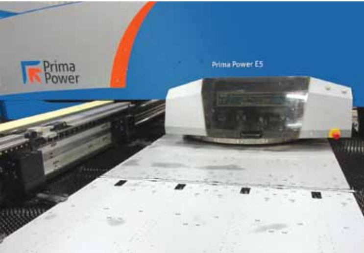
The Prima Power E5 servo electric turret punch press.
