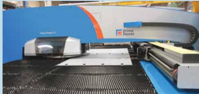
Prima Power says its E5 series turret punch presses offer high performance punching and high accuracy for forming because of the NC-controlled servo-mechanically actuated punching stroke.
