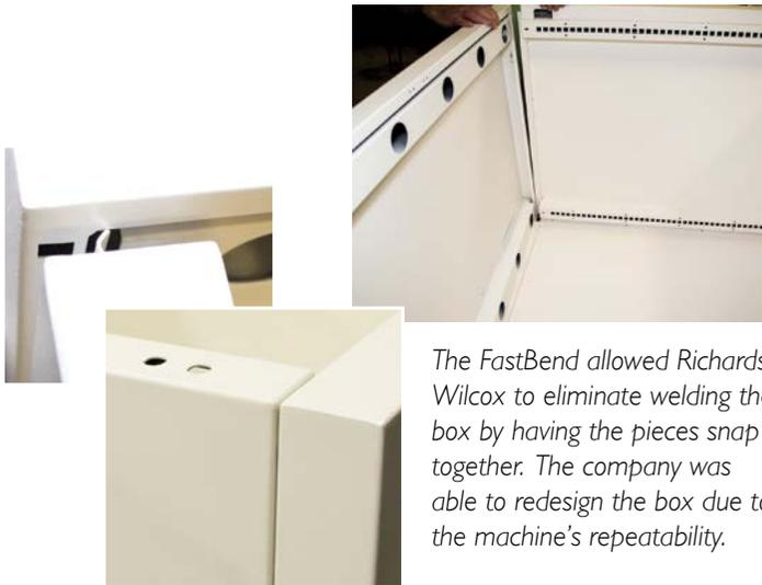
*The FastBend allowed Richards-Wilcox to eliminate welding the box by having the pieces snap together. The company was able to redesign the box due to the machine's repeatability.*
