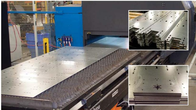
*The addition of the Platino Fiber Laser allowed Richards-Wilcox to save the \$300,000 it was spending on outsourced laser parts. The company went from 2-4 weeks lead times to a one or two day turnaround and offloaded some of its other machines because of the capabilities of the laser.*
