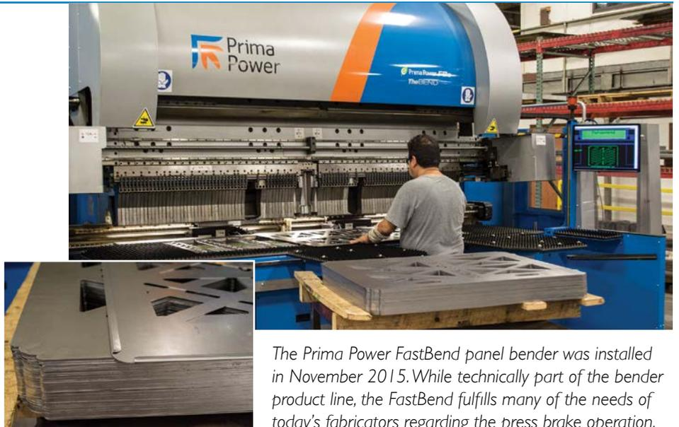
*The Prima Power FastBend panel bender was installed in November 2015. While technically part of the bender product line, the FastBend fulfills many of the needs of today's fabricators regarding the press brake operation.*
