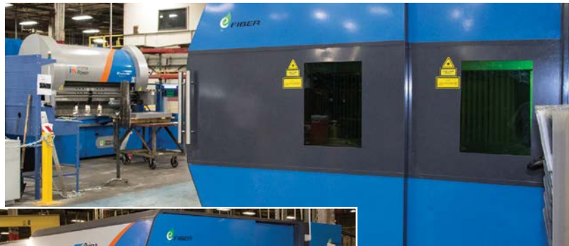
The Platino Fiber cuts various thicknesses, up to 20 mm of mild steel, with efficiency and quality. Productivity increases particularly with thin and medium-gauge sheet metal.
