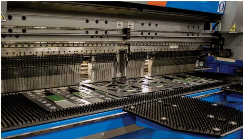
*The FastBend provides a solution to the labor-intensive tool setup, programming, and part handling involved in forming metal in a traditional press brake. It reduces or eliminates non-value added costs associated with the traditional press brake operation. The FastBend operator is simply required to load, rotate, and unload the part.*
