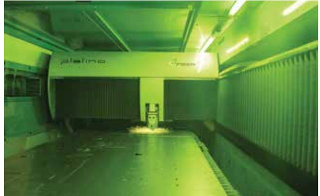
***The Platino Fiber Laser cuts various thicknesses of mild steel up to 20 mm with increasing productivity when cutting thin and medium gauge sheet metal.***
